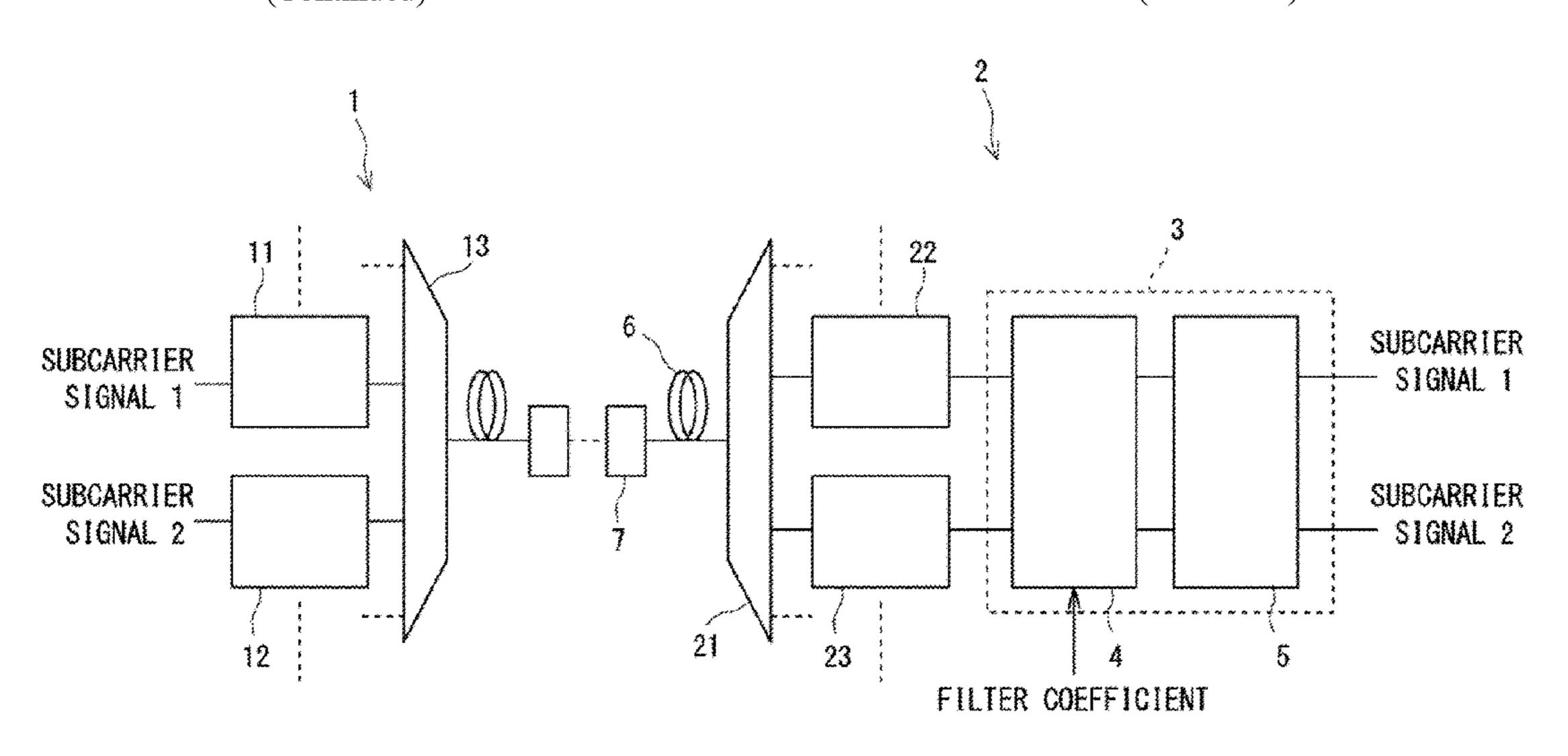
including a FDE-MIMO equalizer (4) and a TDE-MIMO equalizer (5) on each of the separated subcarrier signals.
