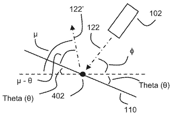
When mirror 110 is tilted to a positive non-zero angle, Theta ( $\theta$ ):
