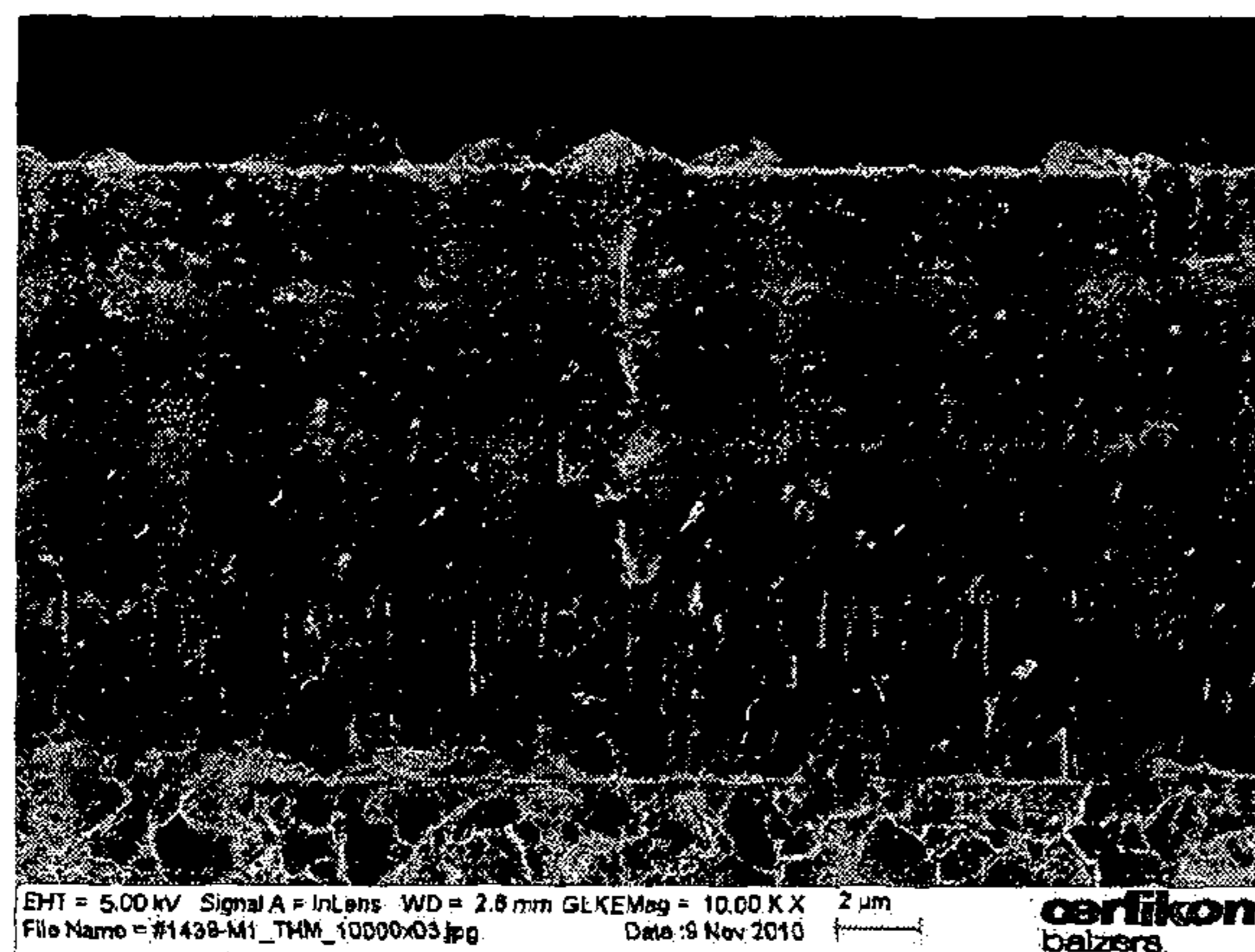
Figure 4: Fracture cross section of the un-polished \text{Mo}_{1.0}\text{N}_{1.0} coating (sample D).
