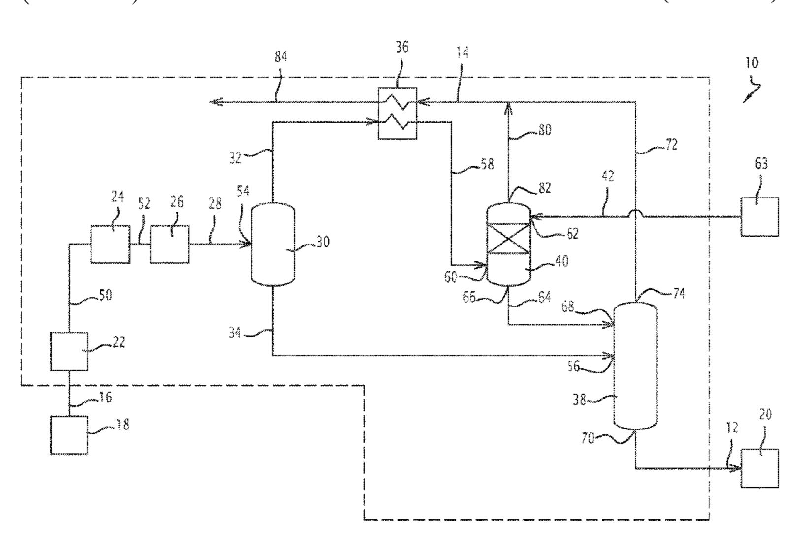
injecting a methane-rich stream into the absorber to place the cooled overhead flow in contact with the methane-rich stream.
