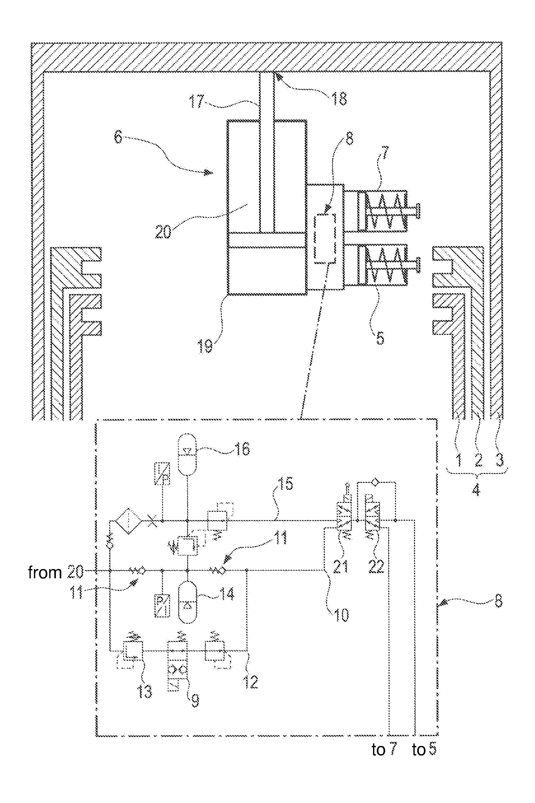
CRANE TELESCOPE LOCKING DEVICE
