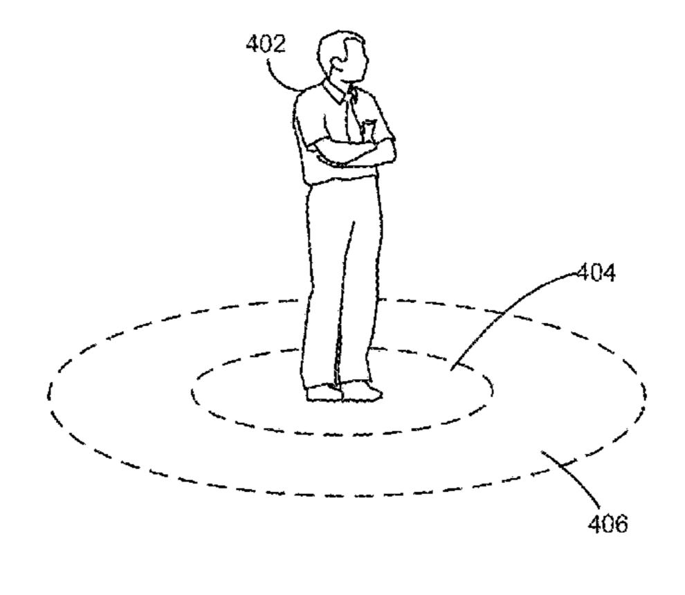
component is configured to provide instructions to the control system to cause the telepresence robot to operate according to a first set of rules when a presence of one or more humans is not detected and operate according to a second set of rules when the presence of one or more humans is detected.
