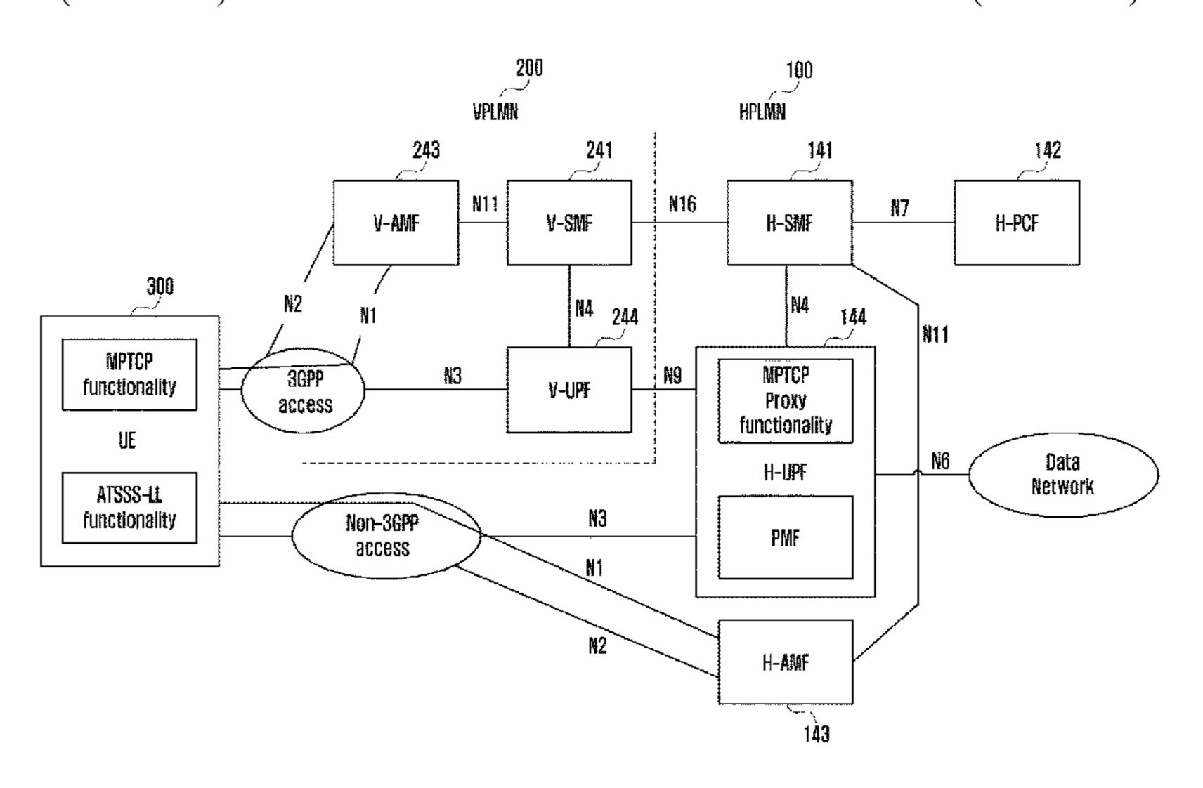
HPLMN-based traffic control in a wireless communication network when a UE 300 is registered on different PLMNs.
