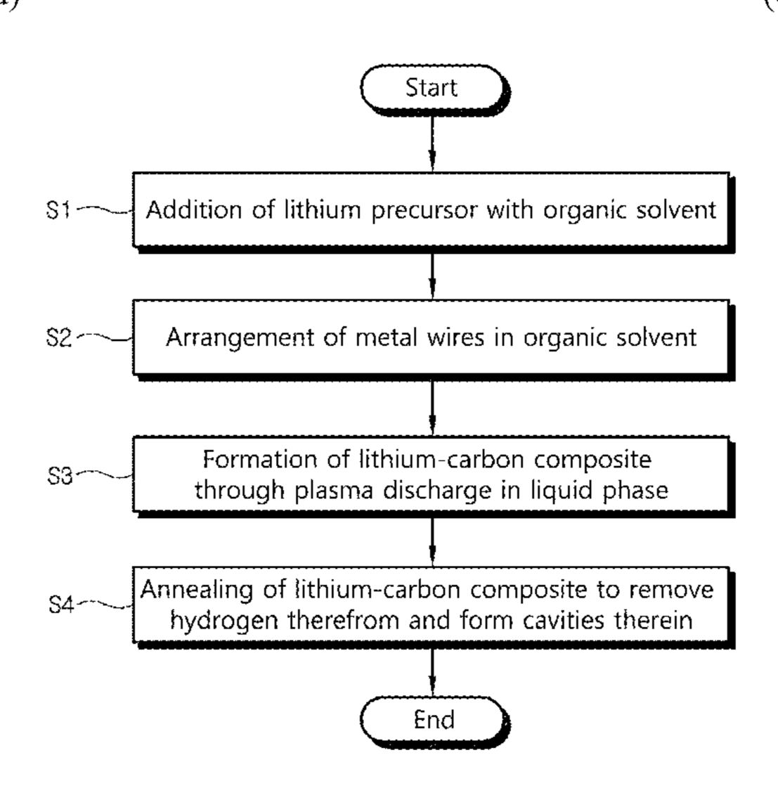
ite and form cavities in the lithium-carbon composite. Accordingly, a lithium-carbon composite can be simply synthesized using plasma discharge in a solution, and the synthesized lithium-carbon composite can be annealed to thus form cavities therein, thereby increasing the lithium charge and discharge performance of a lithium secondary battery using the lithium-carbon composite.
