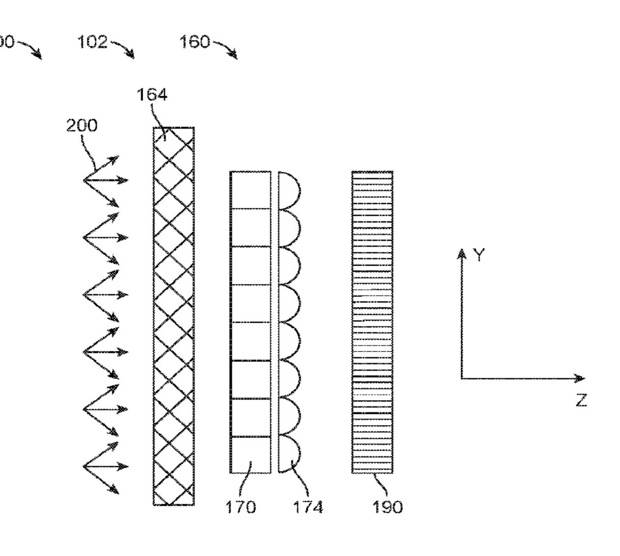
based on an angle of light received at the location, the focal length of the lens and the central wavelength of the filter.
