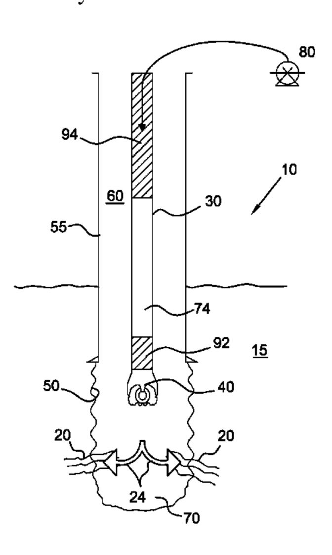
injecting the remainder into the tubular element, until it comes into contact with the fluid injected through the annulus to form a blocking polymer at the thief zone.
