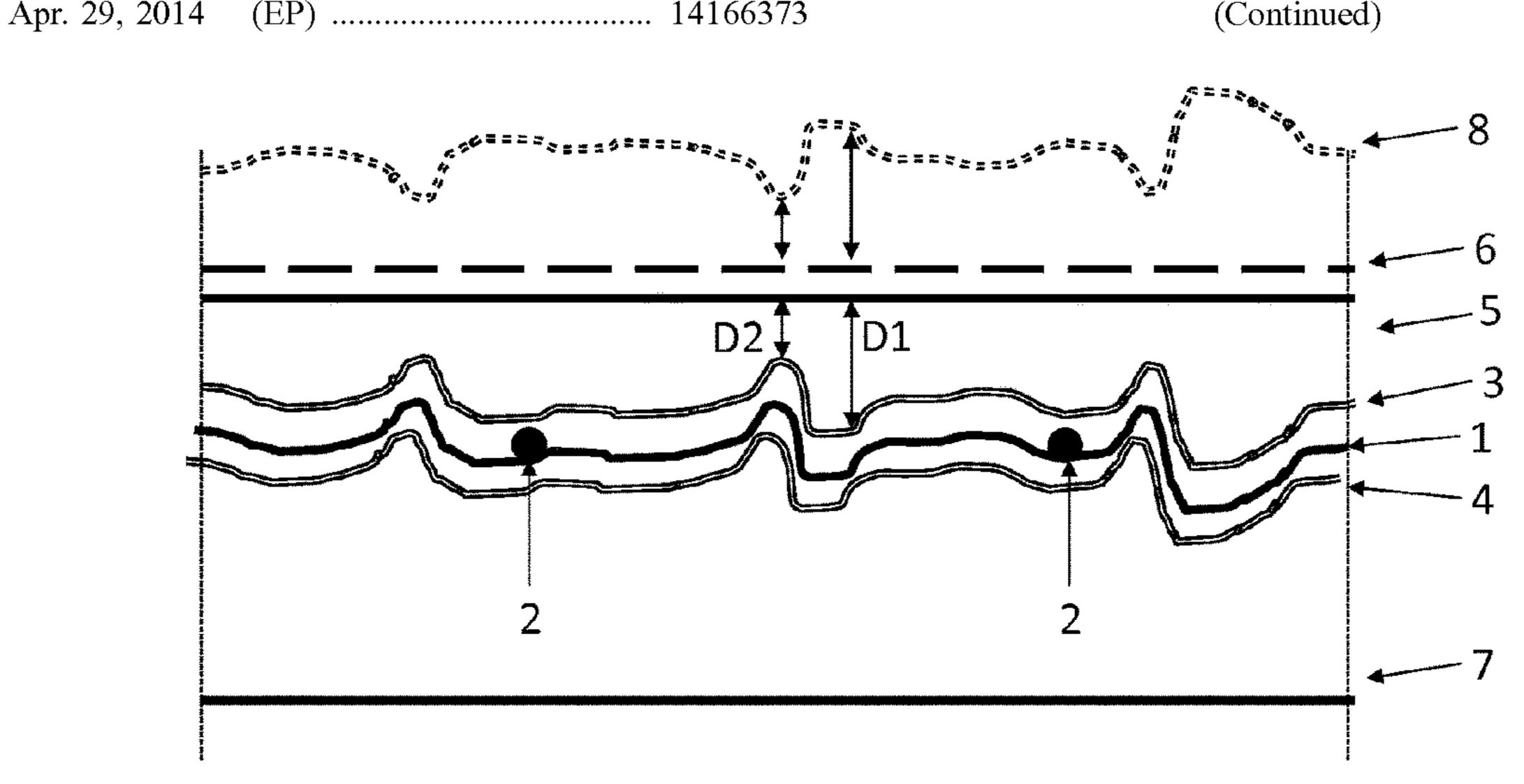
The carrier material prevents the formation of surface irregularities and printing errors in the vinyl floor covering.
