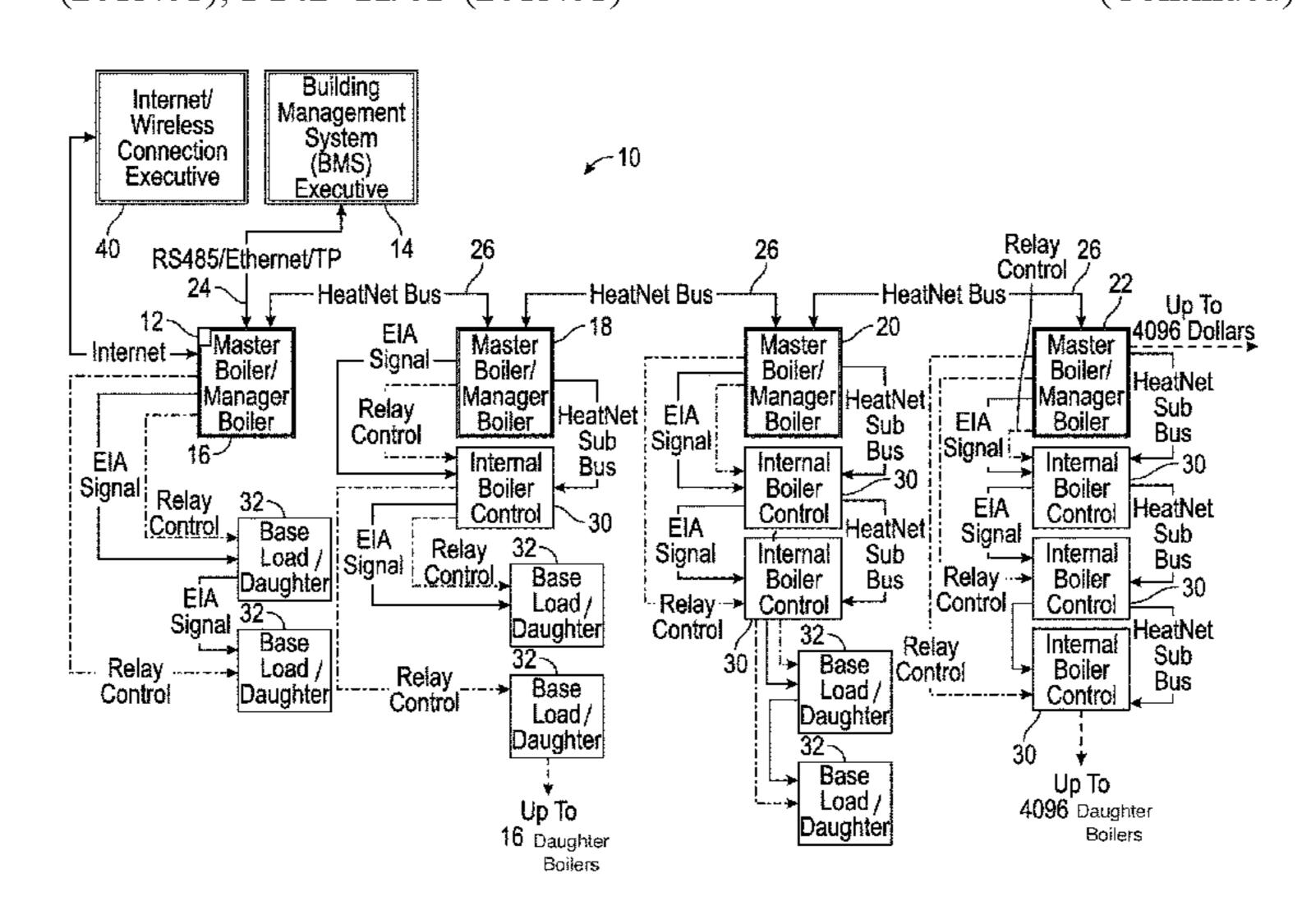
boiler including a plurality of nested sub boilers; connecting the first boiler to an external control; and with a boiler control connected to one of said first boiler and said at least one secondary boiler, controlling a boiler parameter of said first boiler, said at least one secondary boiler, and said plurality of nested sub boilers of said at least one secondary boiler.
