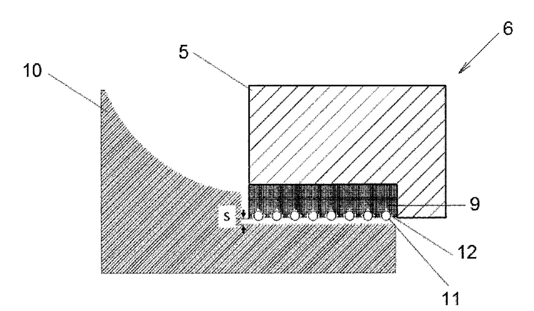
the rotating and non-rotating elements when the sealing gap is reduced. The elements and the bodies may be formed in an additive manufacturing process.
