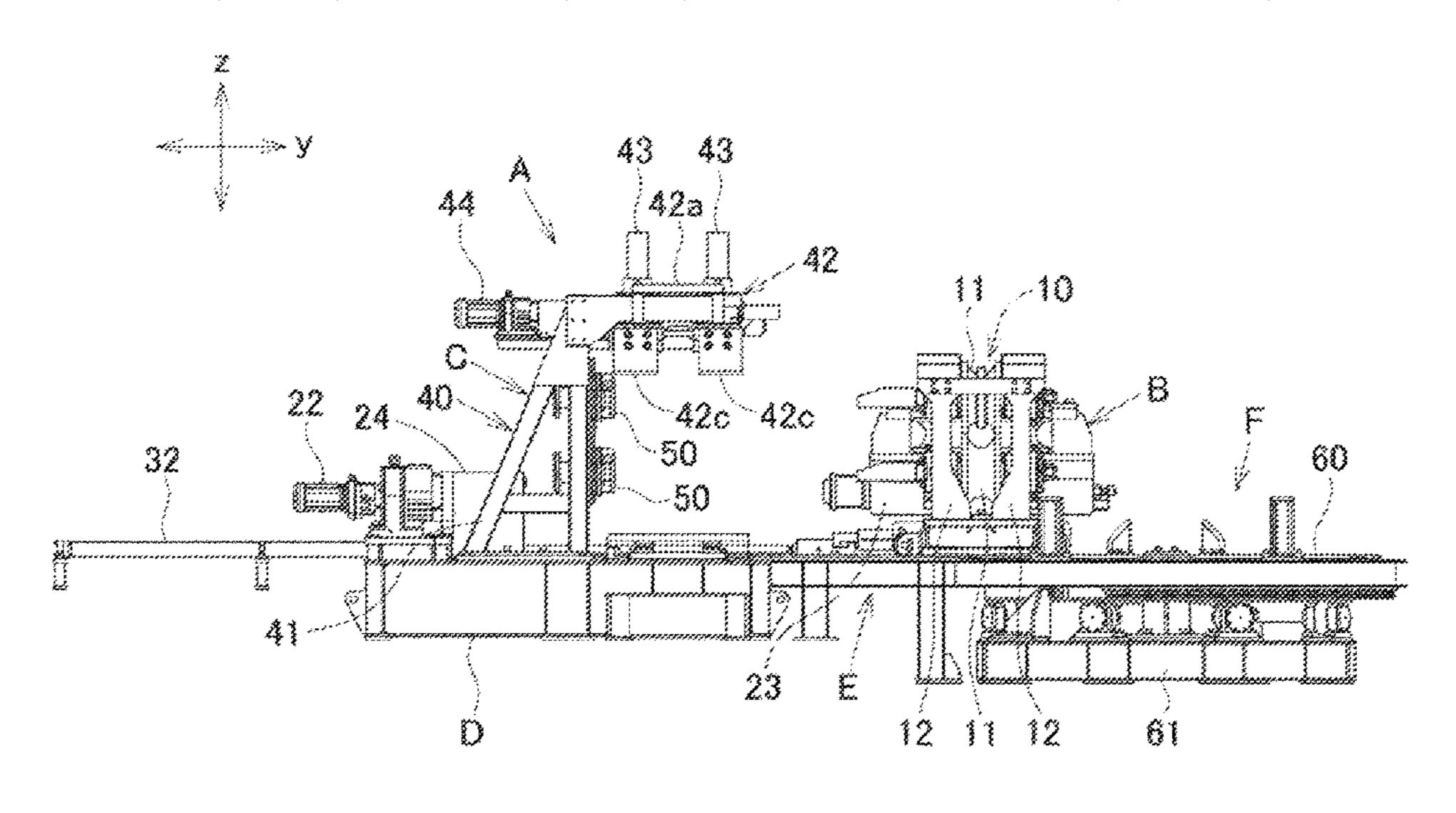
the opened top, and retreats to the outside of the forming line while the pressure device 43 is left on the forming line. The overhang part 42 of the fixed stand 40 is engaged with the horizontal roll housing 12 of the horizontal roll stand 10 to support the horizontal roll housing 12 in the forming line.
