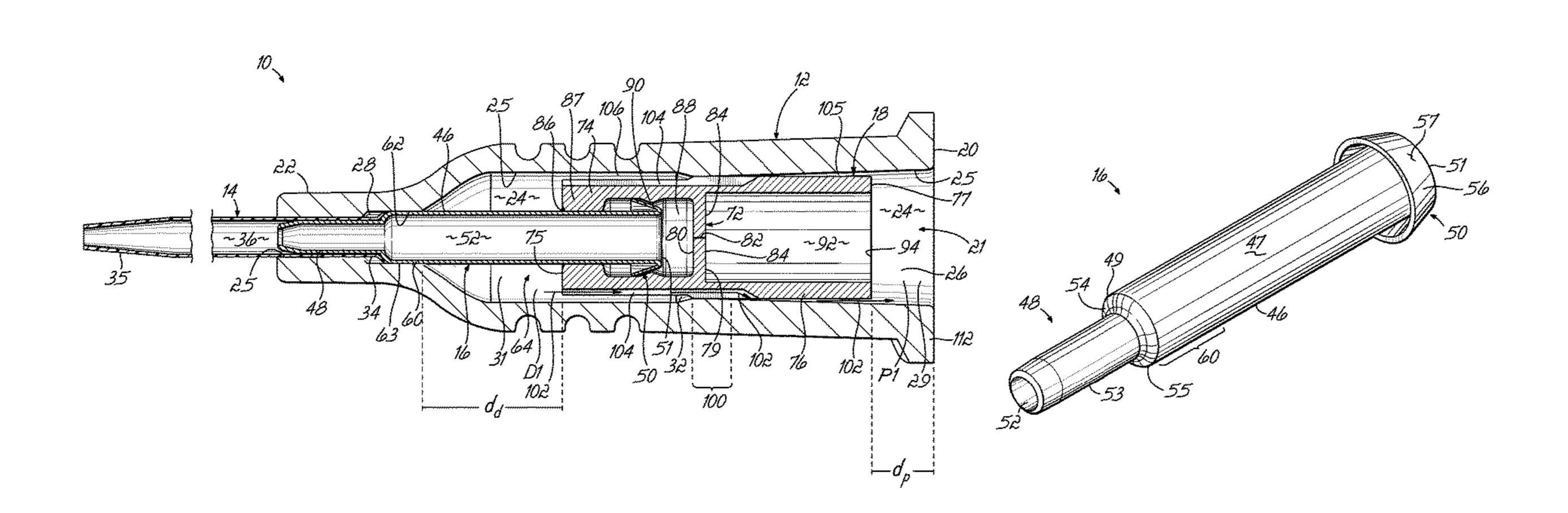
biasing member that moves the seal member to force the membrane back over the actuator to close the membrane.
