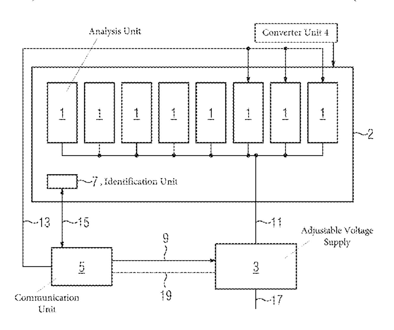
able voltage supply to equate the provided supply voltage to the operating voltage of the at least one analysis unit.
