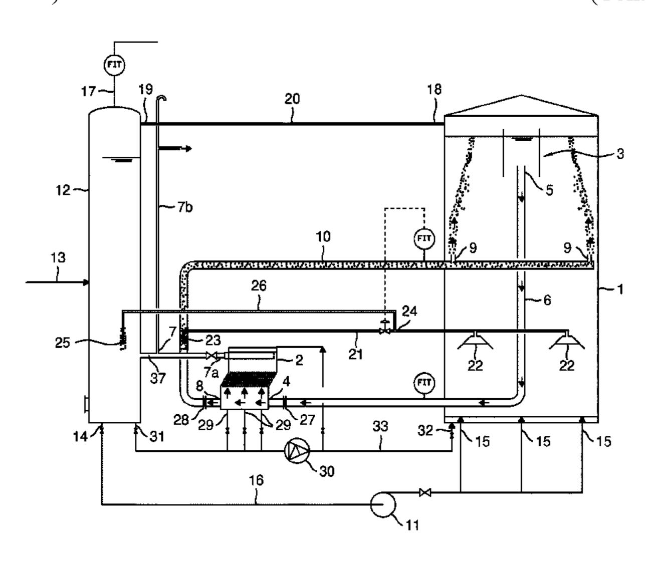
separator, wherein the aqueous fluid that includes the biomass is separated into a liquid phase and a fluid phase enriched in biomass; returning the fluid phase enriched in biomass from the external separator to the bioreactor; and returning a part of the liquid phase to the conditioning tank.
