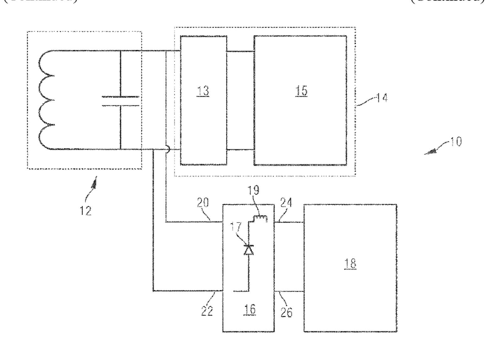
first rectifier output is coupled to an output of the rectifying element and to the first rectifier input by a first inductor.
