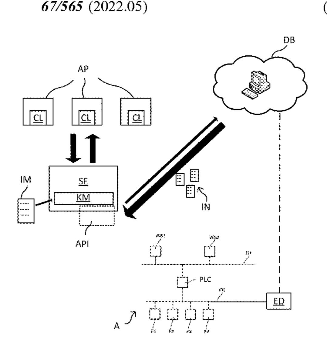
database using the API and transferring the information from the API to the OPC UA server; converting the queried information into OPC UA-conforming structure data; and sending the structure data from the OPC UA server to the OPC UA client.
