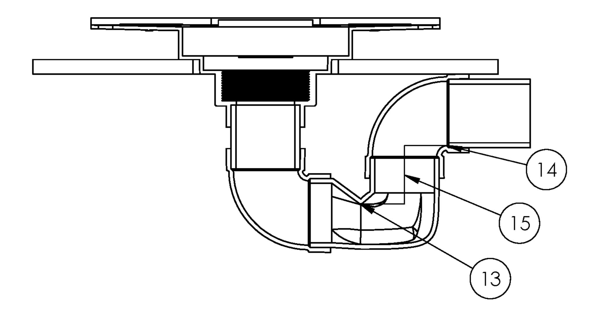
Flg. 4. Cross-section of trap showing weir height.
