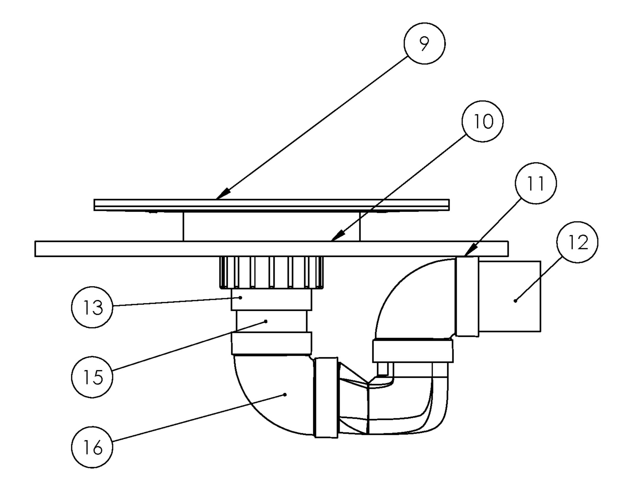
Flg. 3. Lateral view of trap attached to drain through subfloor.
