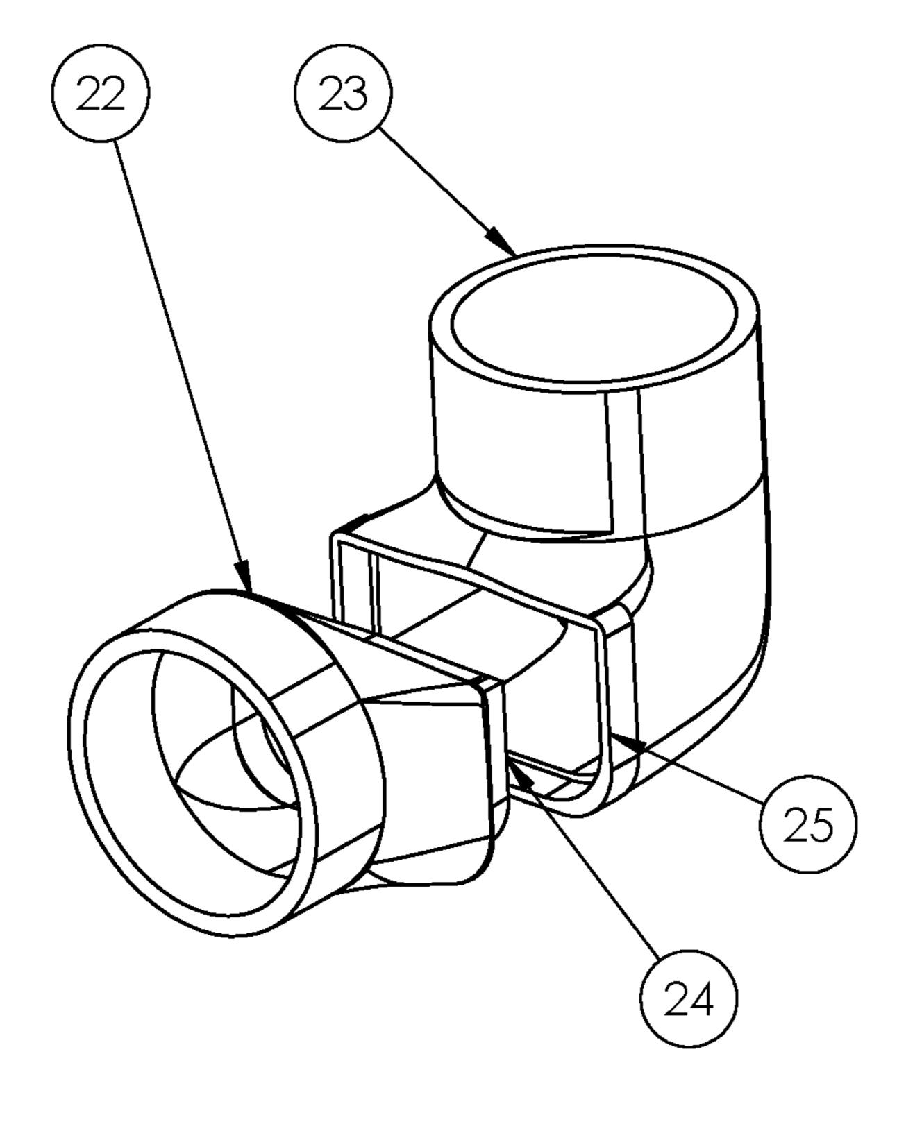
Flg. 6. Exploded isometric view of flattened elbow.
