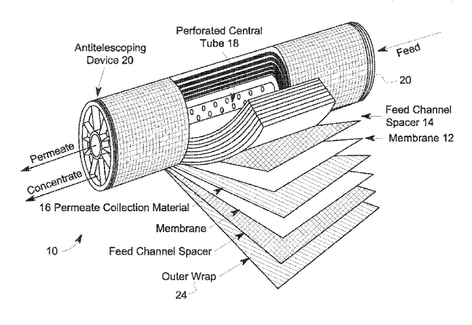
module may be used at a temperature of up to 130° C. Optionally, the module may be used at a pH of 9.5 or more. In a filtration method, the module may be operated at a pressure in the range of 150 to 450 psi. The module may be operated at a generally constant pressure.
