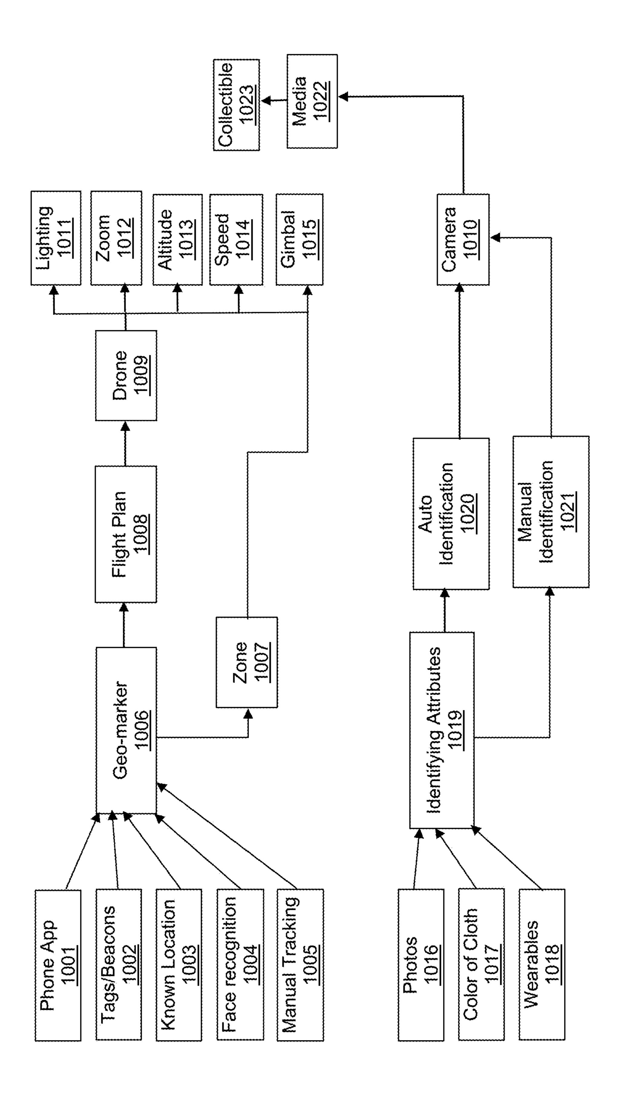
Fig. 1: Flow Diagram - Capture Location & Photos / Videos
