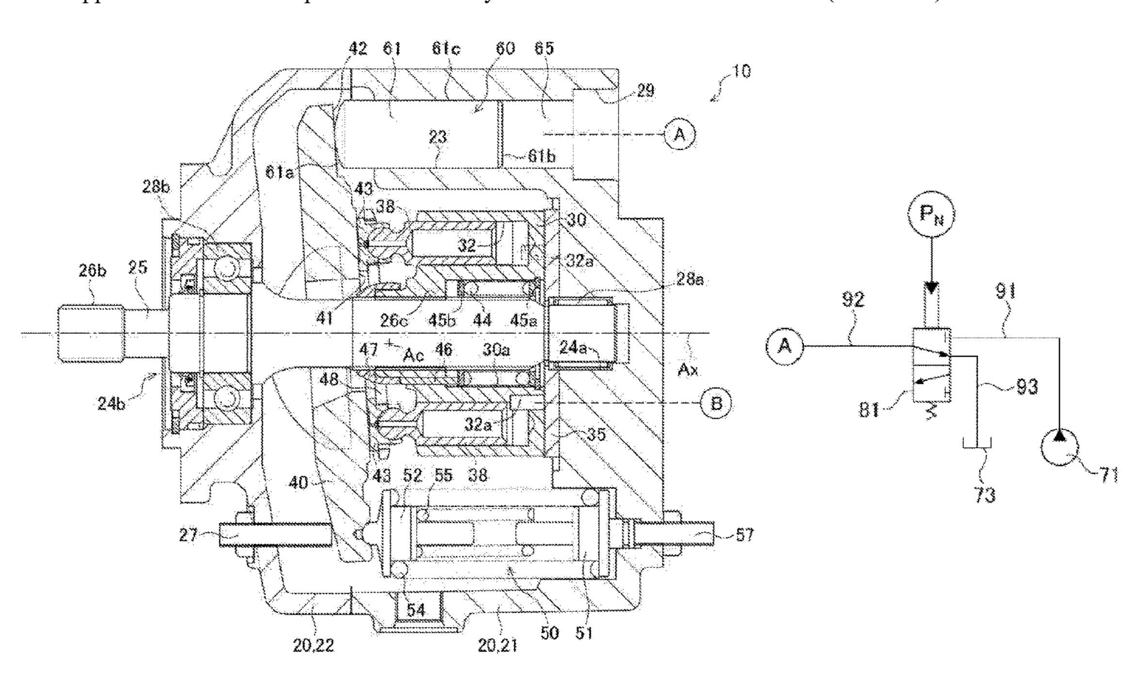
pressing the swash plate in such a direction as to increase the tilt angle of the swash plate by a pressure supplied from the outside of the hydraulic pump.
