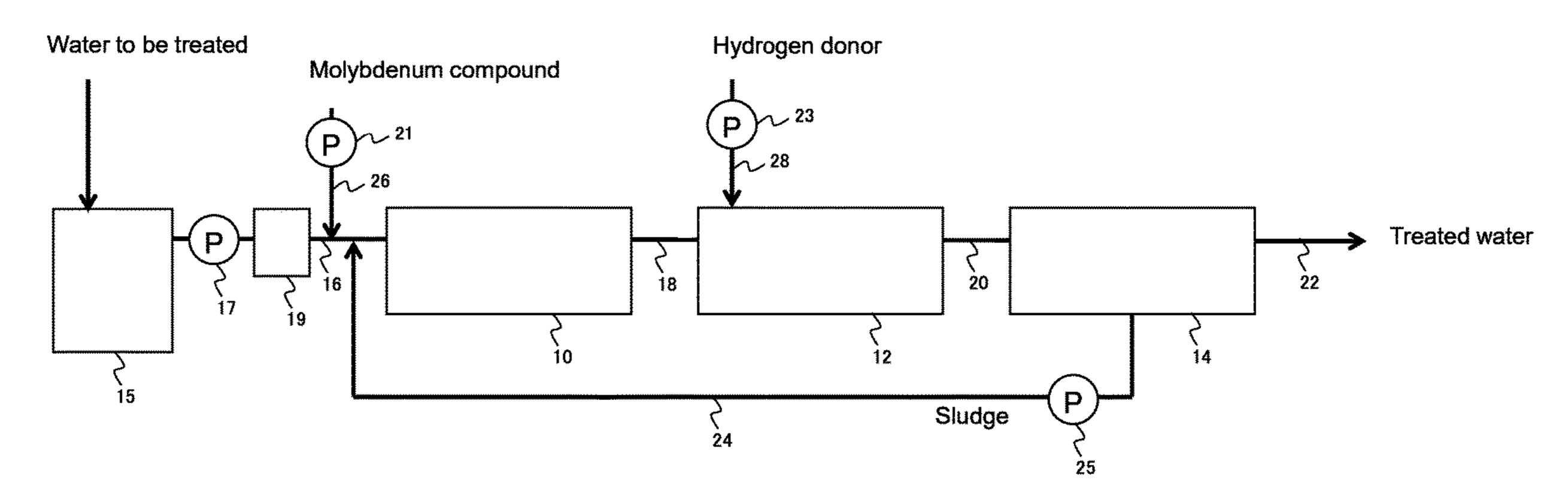
vated sludge; and a nitrification rate control means which maintains a molybdenum compound in the nitrification device in such a manner as to control the molybdenum concentration of the water to be treated to 0.025 mg Mo/gN or more, and controls the nitrification rate for the sludge to 0.11 [kgN/(kgVSS·day)].
