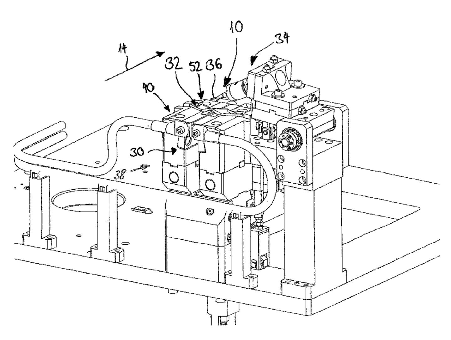
invention, the hard material element (4) can be centered relative to the centered and fixed saw blade (8) by means of the second centering device (32), and the first and second centering device (30) are provided in a common assembly (38), such that the centering of the saw blade (8) by the first centering device (32) predetermines a centering position for the subsequent centering of the hard material element (4) by the second centering device (32).
