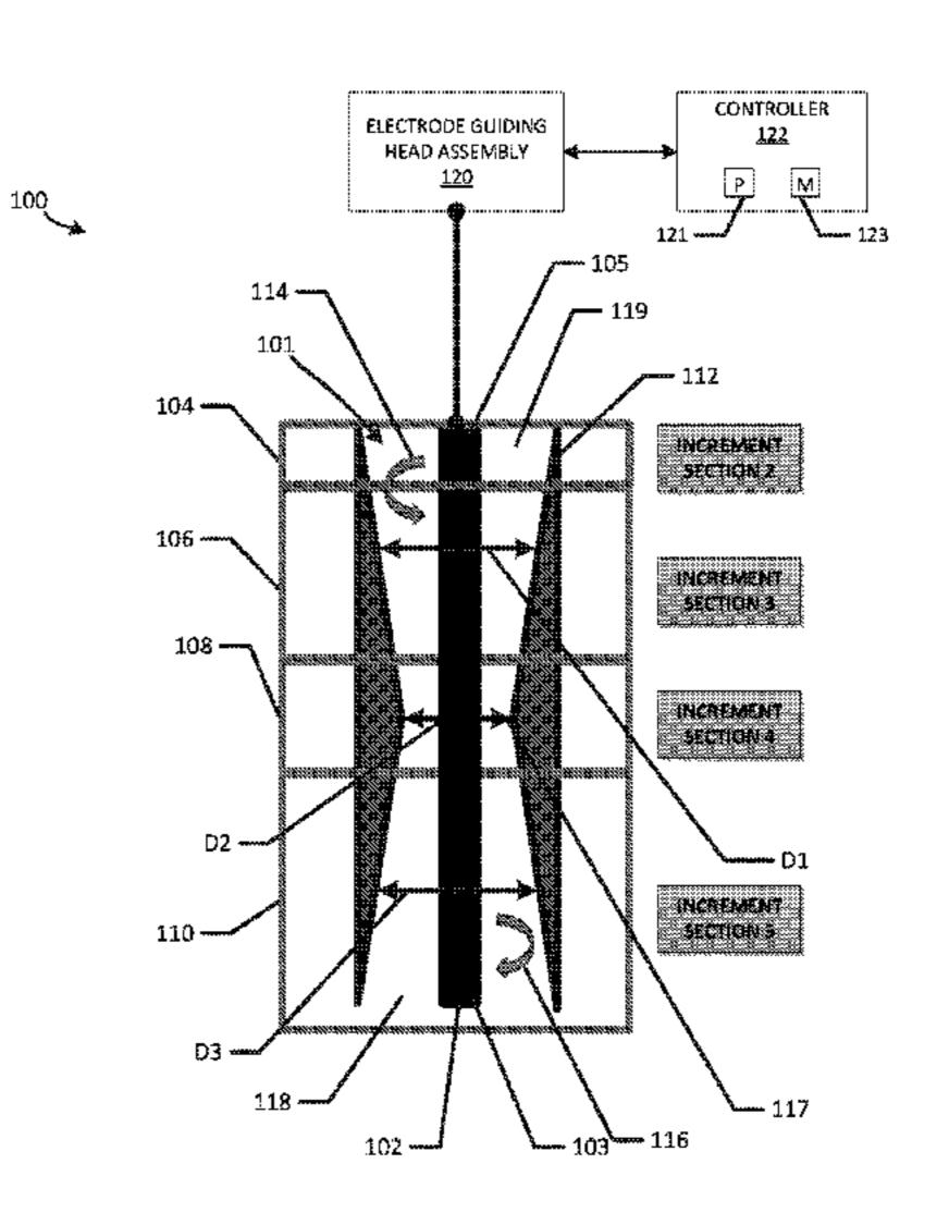
distance wherein advancing the electrode and applying the second voltage causes formation of at least a second orifice section; wherein the first and second orifice sections cooperate to form an orifice comprising a first flow area and a second flow area.
