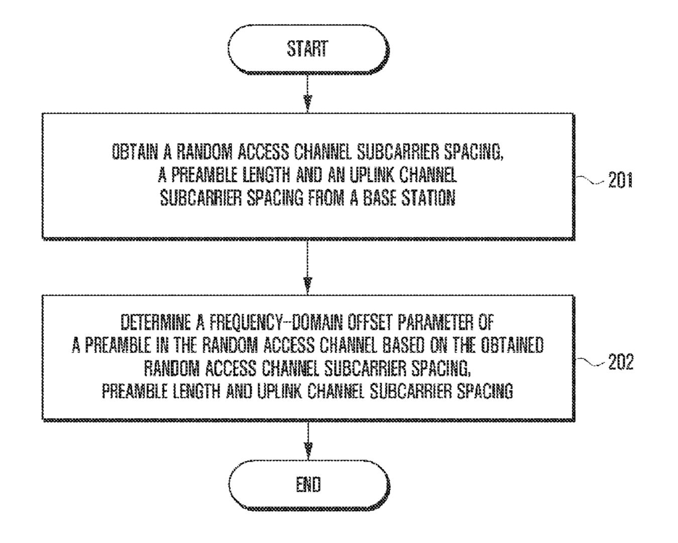
station and determining a frequency-domain offset parameter  $\bar{k}$  of a preamble in a random access channel based on the obtained random access channel subcarrier spacing  $\Delta f_{RA}$ , preamble length  $L_{RA}$  and UL channel subcarrier spacing  $\Delta f$ . Other embodiments of the disclosure further provide a random access method, a method for configuring random access information and related device, and a corresponding computer readable medium.
