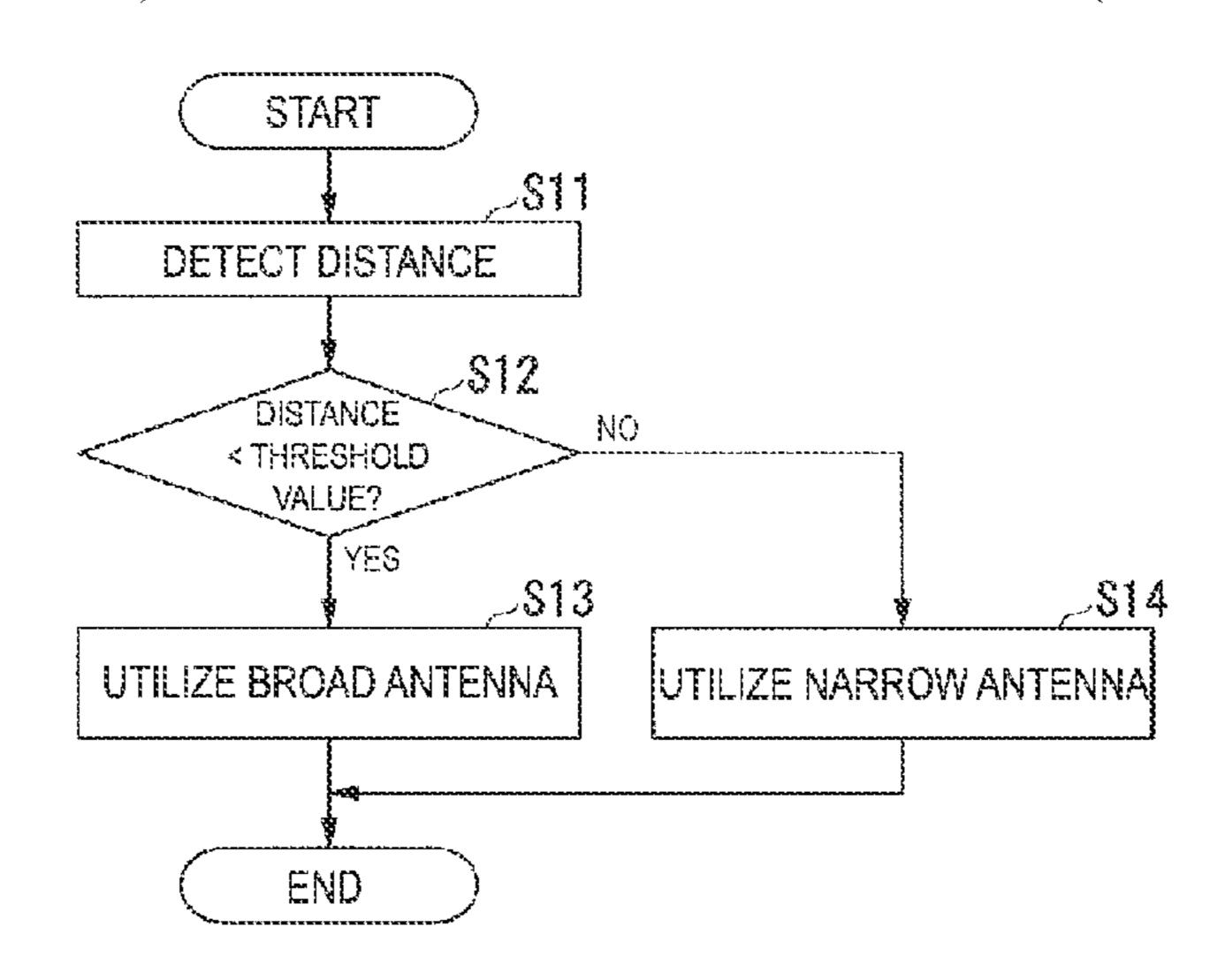
width of an electromagnetic wave emitted from the first mobile station to the second mobile station the distance.
