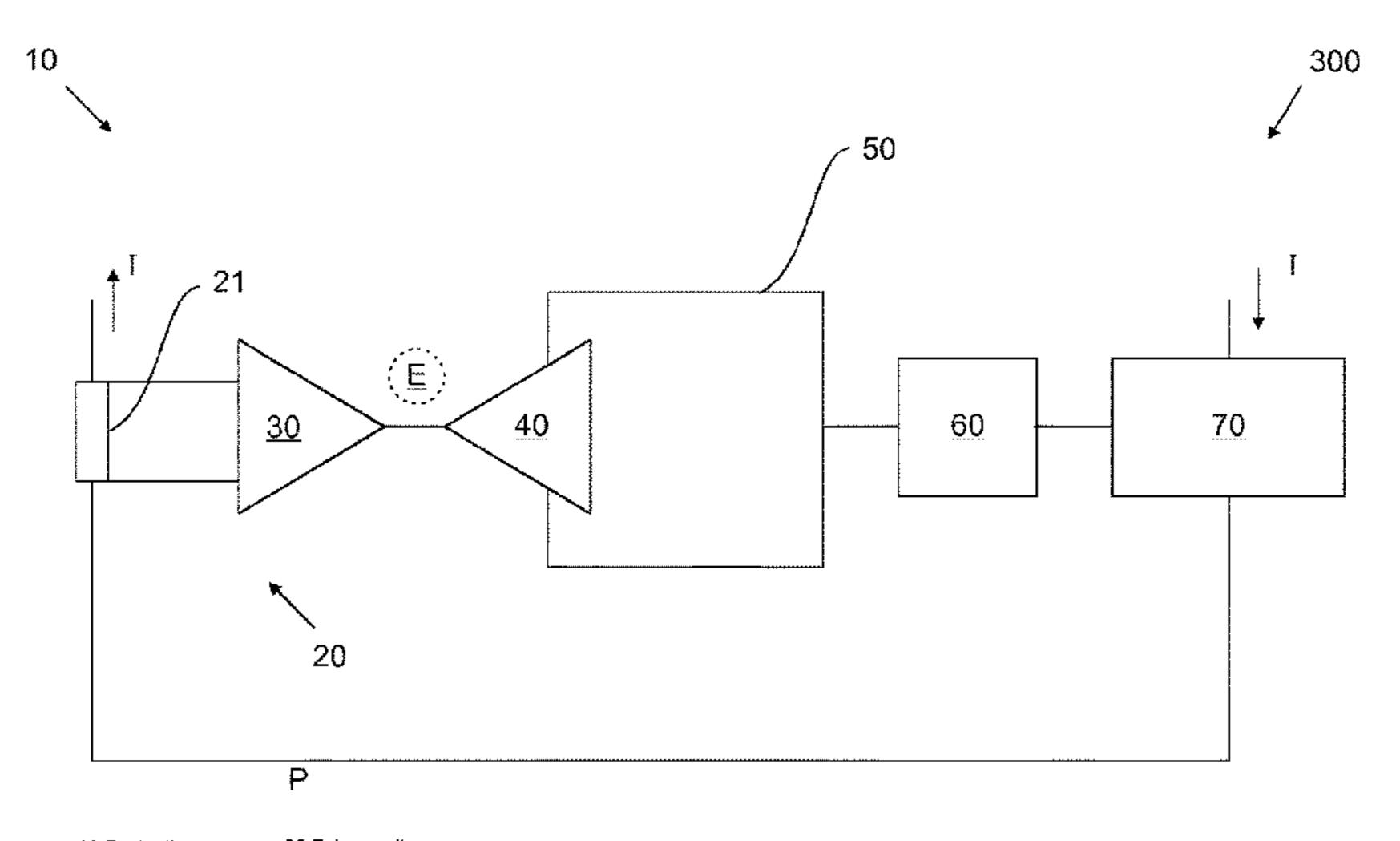
10 Protection system 60 Driver unit 70 Protection element 20 Acquisition unit
