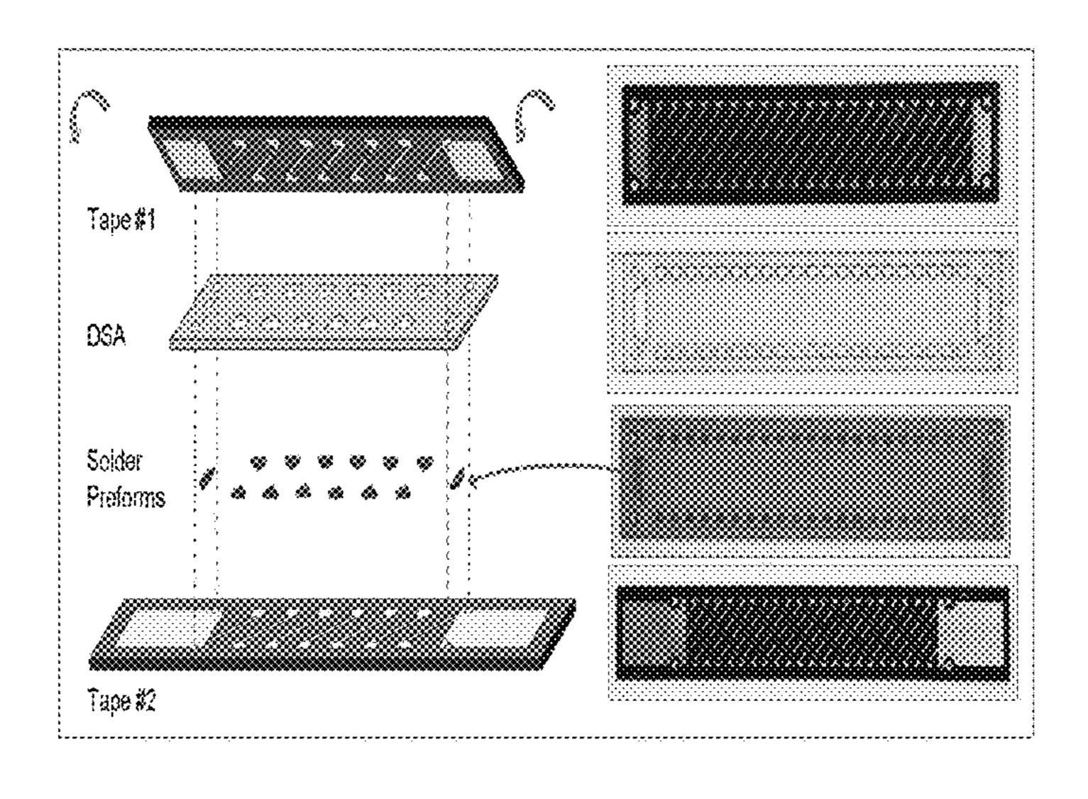
separate tapes to form a single tape structure makes it compatible with a reel-to-reel production process.
