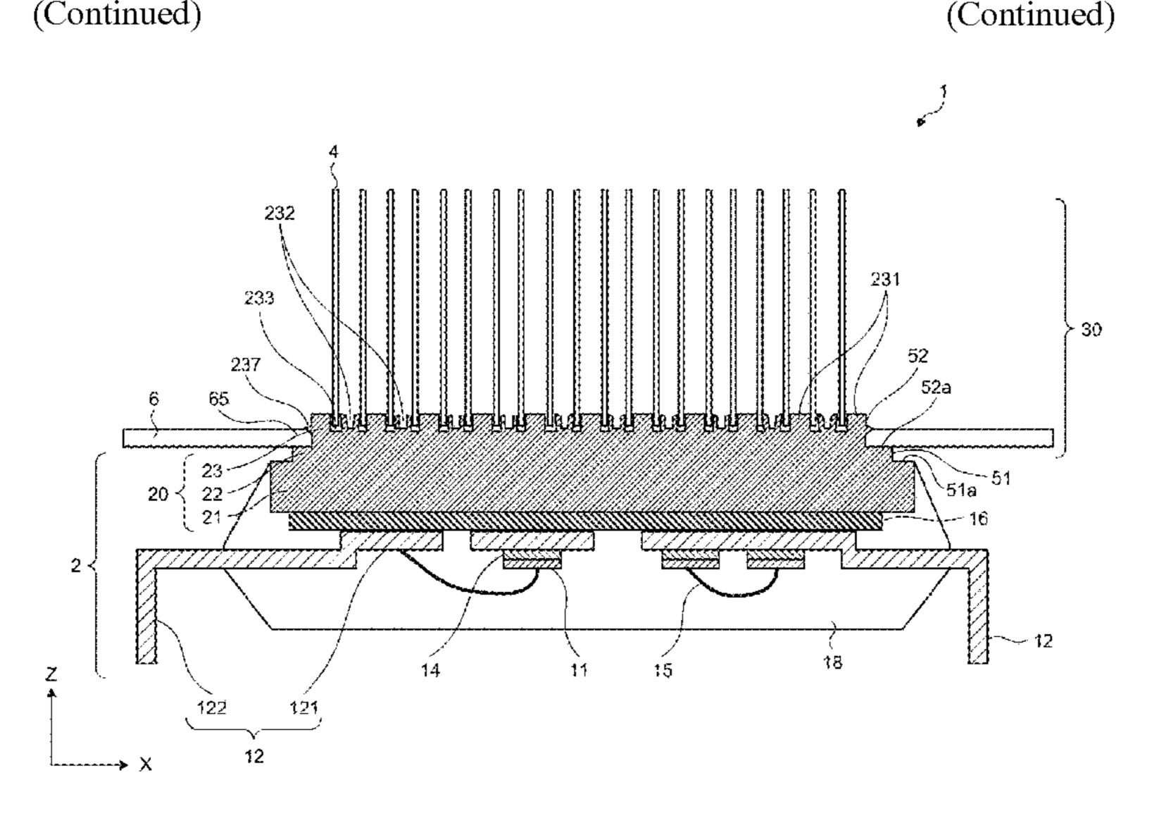
has cover portions covering the fifth surfaces, and is plastically deformed to allow the panel to be fitted in the base plate to fill gaps.
