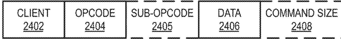
FIG. 24B GRAPHICS PROCESSOR COMMAND SEQUENCE
