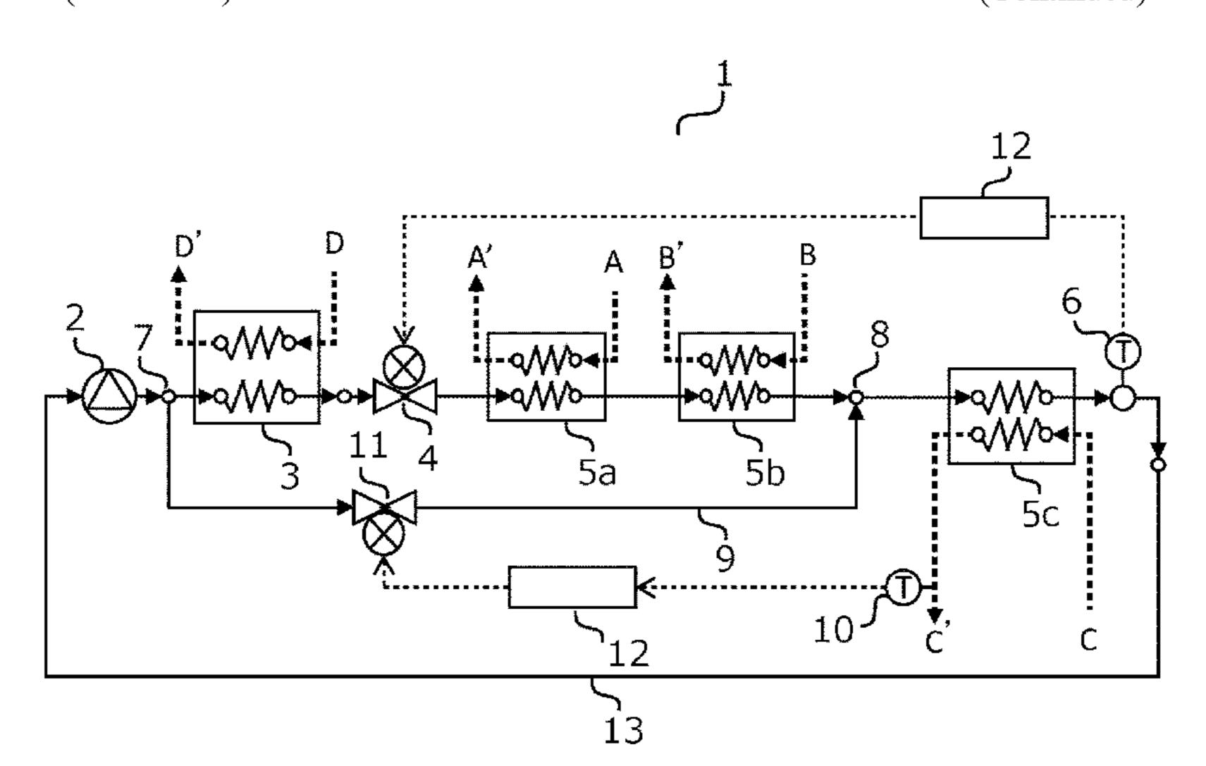
first decompressor depending on the temperature and/or the pressure detected by the detection unit.
