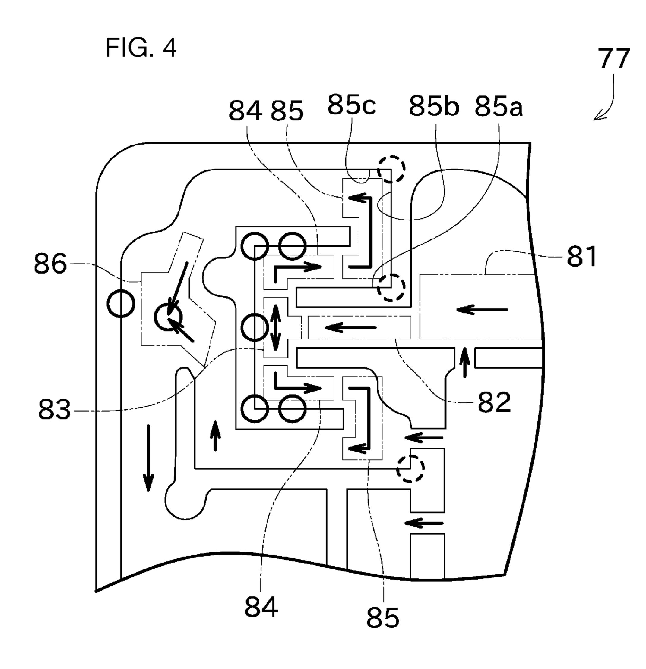
POSITION WHERE ENGINE OIL MIST HAVING LARGE PARTICLE DIAMETER IS LIKELY TO BE SEPARATED
