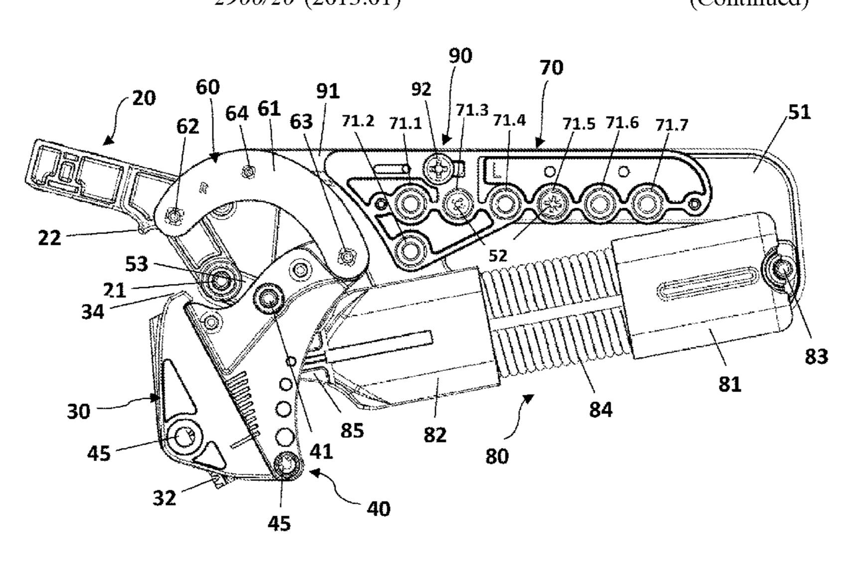
arm; a damping element located on said lever arm for damping the furniture door that is being closed over the furniture body; and a damping adjustment on said lever arm for the purpose of changing the position of a cylinder belonging to the damping element with respect to the lever arm.
