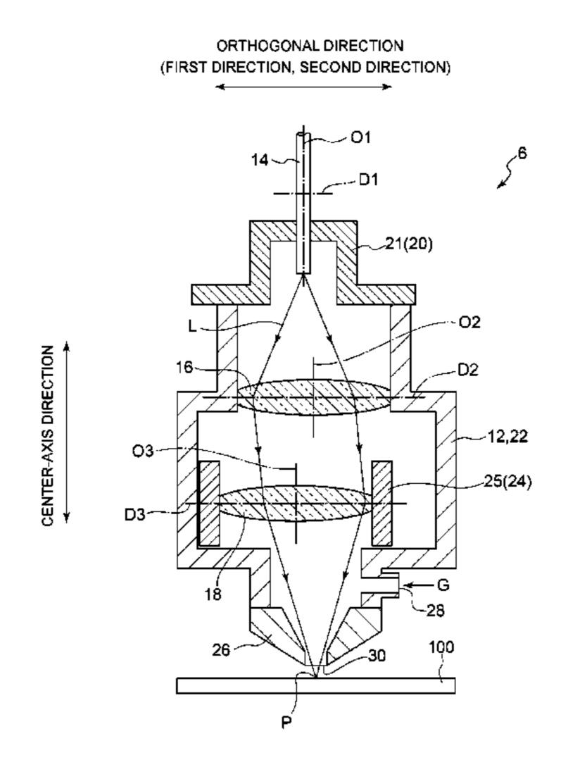
tem, in a second direction orthogonal to a center axis of the collecting optical system.
