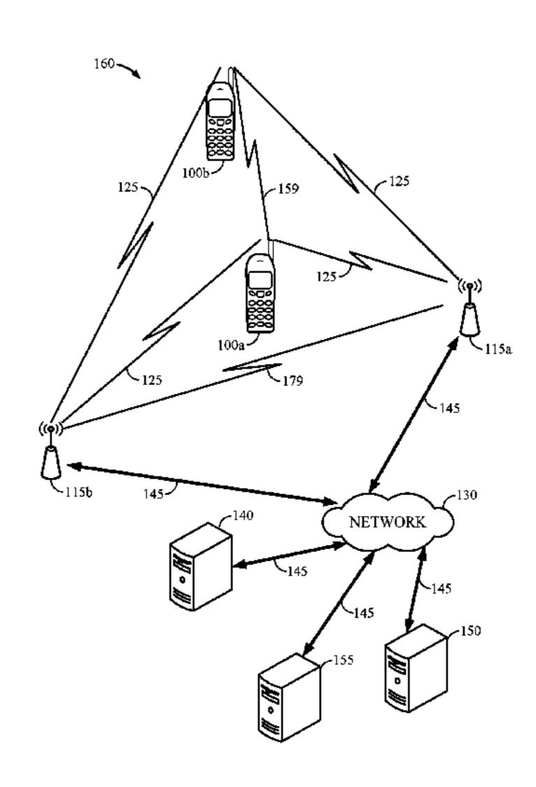
messages from a responding wireless station. An acknowledgement messages may be transmitted to the responding wireless station in response to receipt of the FTM message.
