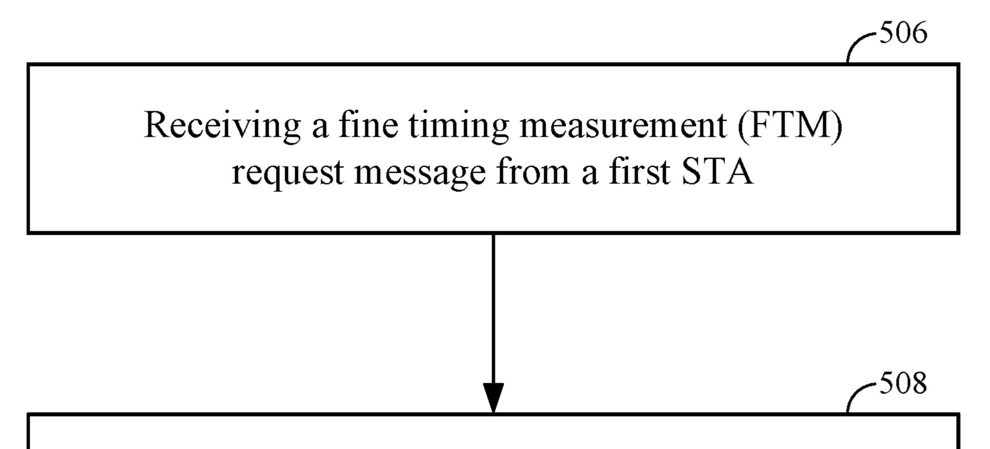
Transmitting at least a clear to send message in response to the FTM request message, the clear to send message comprising one or more parameters specifying a duration of time that the second STA and the first STA are to exclusively occupy a wireless communication medium for the transmission of messages between the second STA and the first STA
