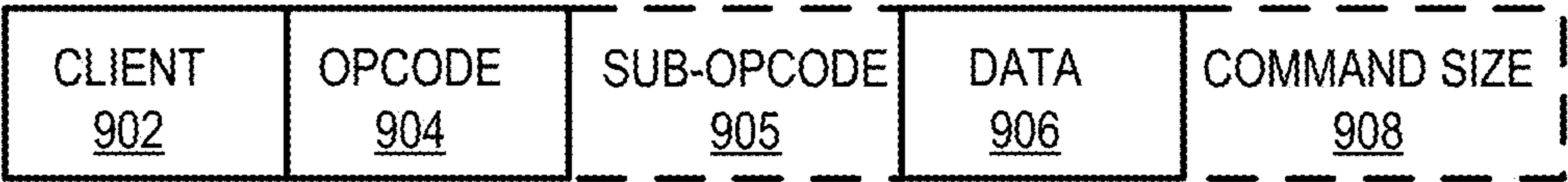
FIG. 9A GRAPHICS PROCESSOR COMMAND FORMAT 900
