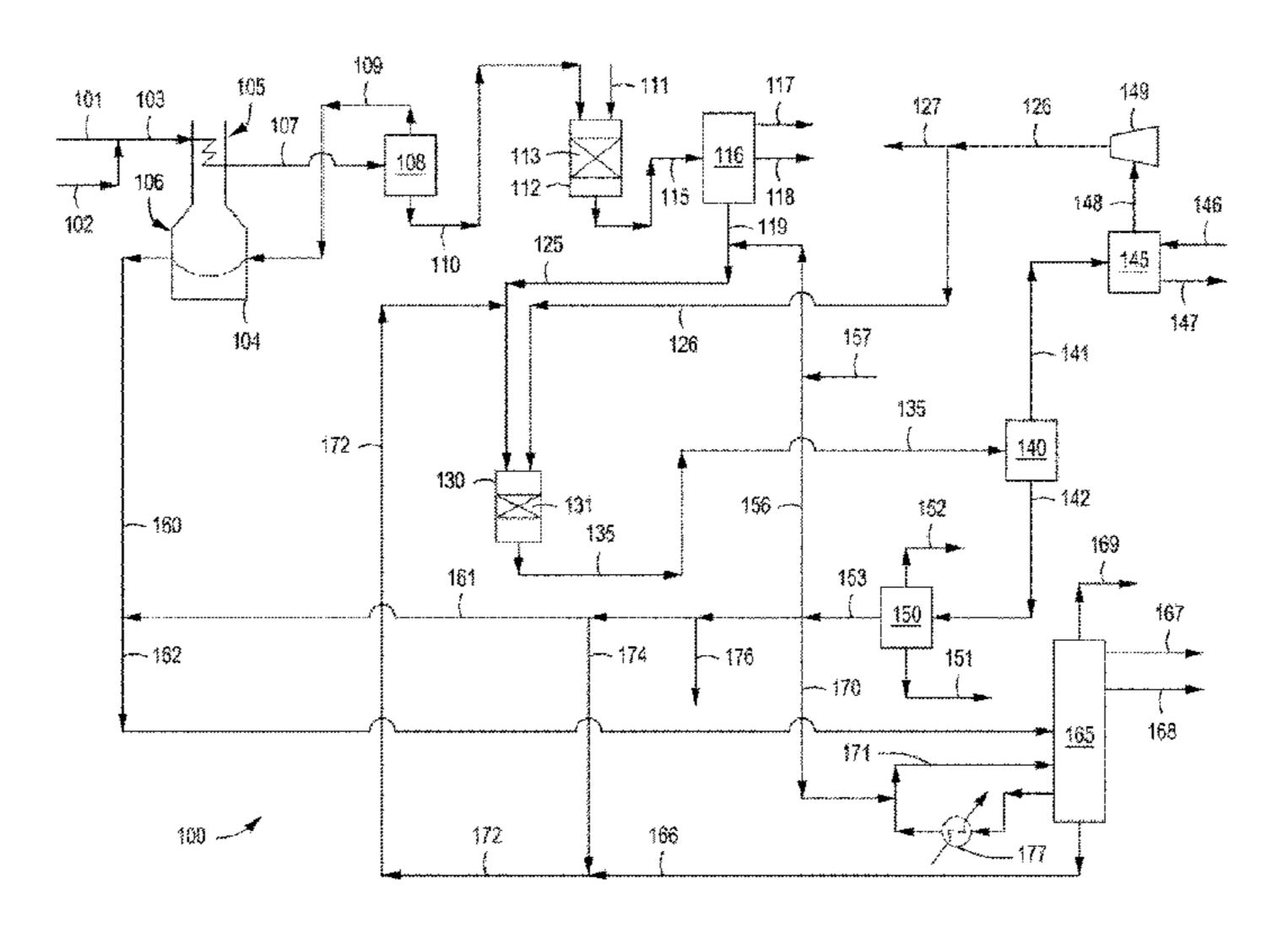
ethylene and propylene can be separated from the steam cracker effluent.
