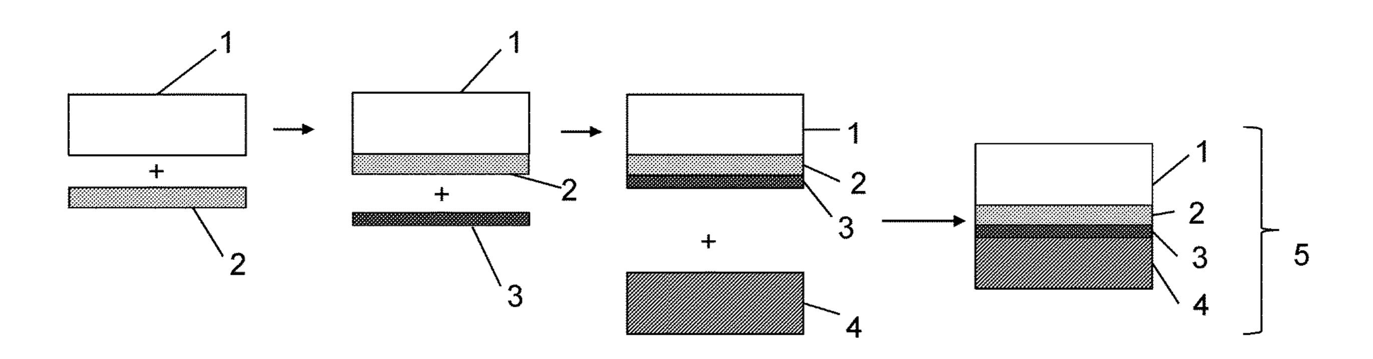
the ink composition, the further composition and the crosslinker are disposed between the first and second flexible substrates.
