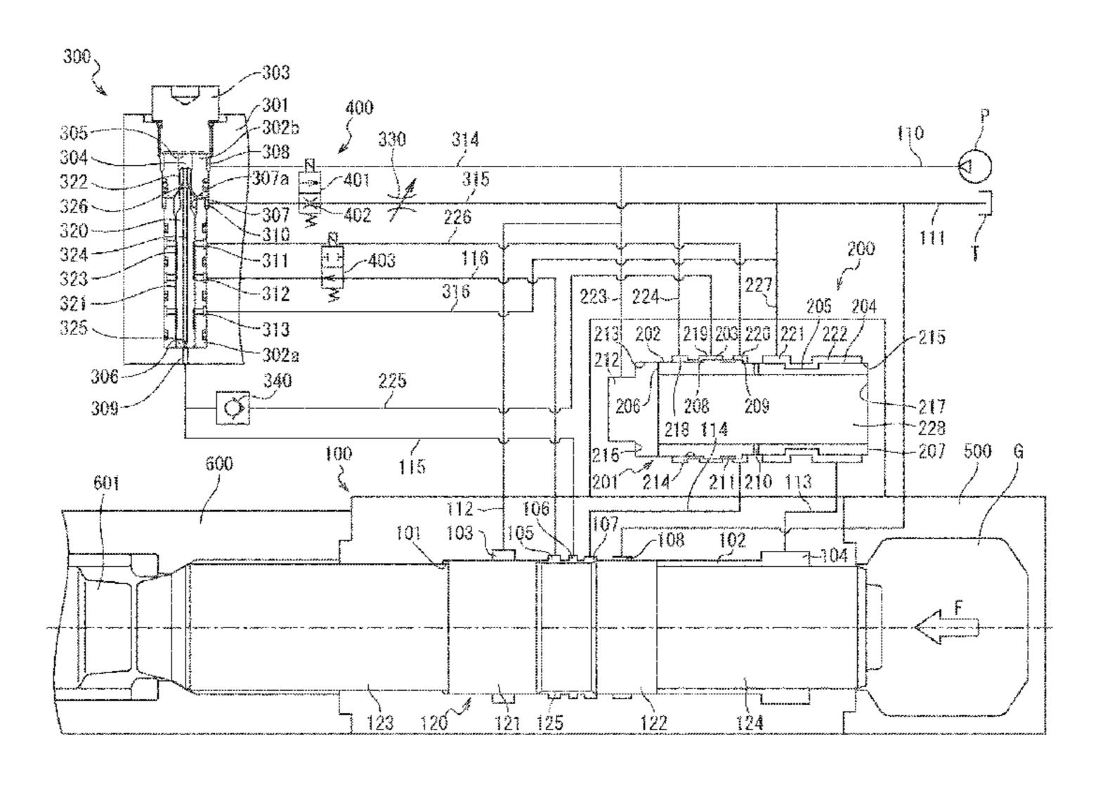
selected. When prohibiting supply of pressurized oil to the auto-stroke setting portion and allowing discharge of pressurized oil from the idle strike prevention setting portion, the idle strike prevention mode is selected.
