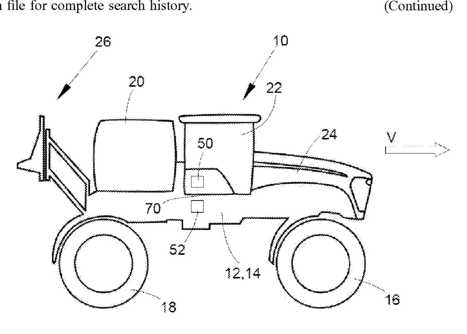
dent on the input variables and configured to drive the actuator on with a view to maintaining the positions of the booms in a desired position above the field contour wherein due to the mechanical coupling of the pair of booms by the middle segment, also results in a movement of other respective booms.
