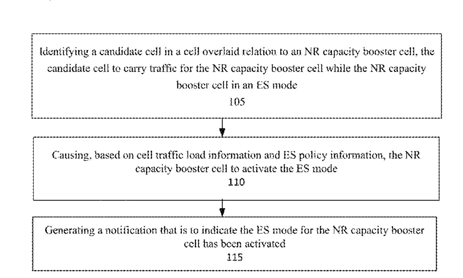
Identifying a candidate cell in a cell overlaid relation to an NR capacity booster cell, the candidate cell to carry traffic for the NR capacity booster cell while the NR capacity booster cell in an ES mode
