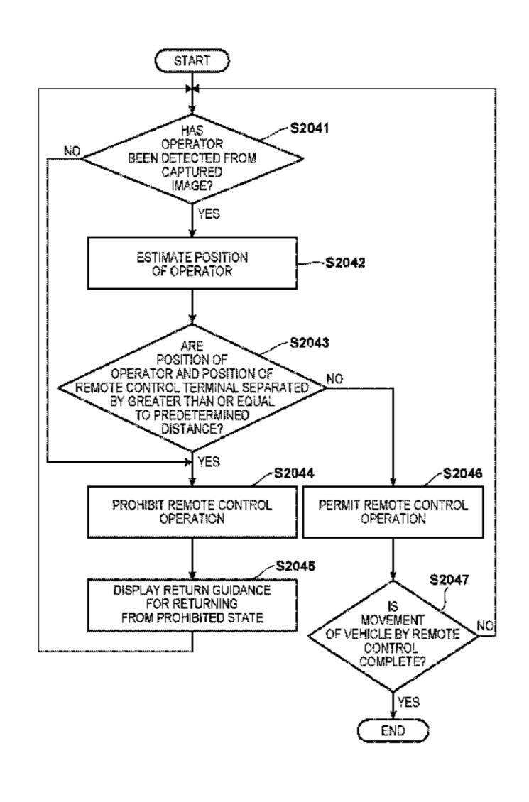
prohibit a remote control operation of the vehicle performed through the remote control terminal.
