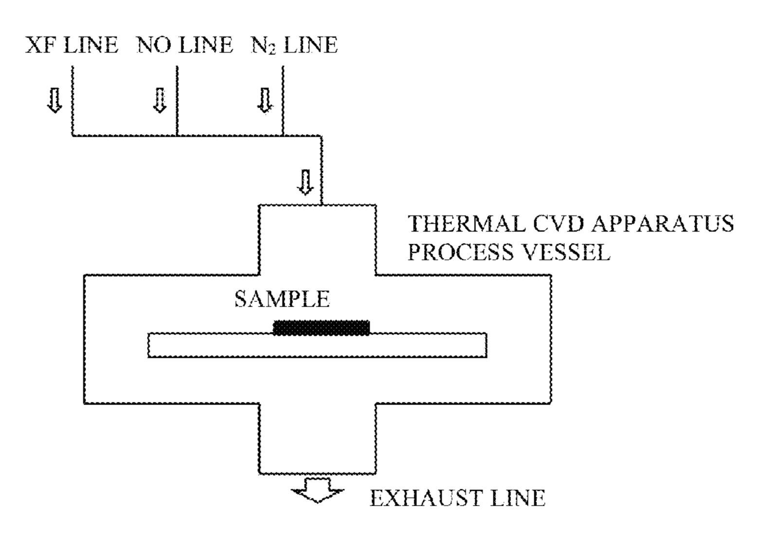
by thermal excitation, it is possible to selectively and rapidly etch a Si-based film, such as Poly-Si, single crystal Si, or a-Si, while decreasing the etching rate of SiN and/or SiO<sub>2</sub>. It is also possible to perform cleaning by removing a Si-based deposited and/or attached matter inside a film forming apparatus, such as a CVD apparatus, without damaging the apparatus interior.
