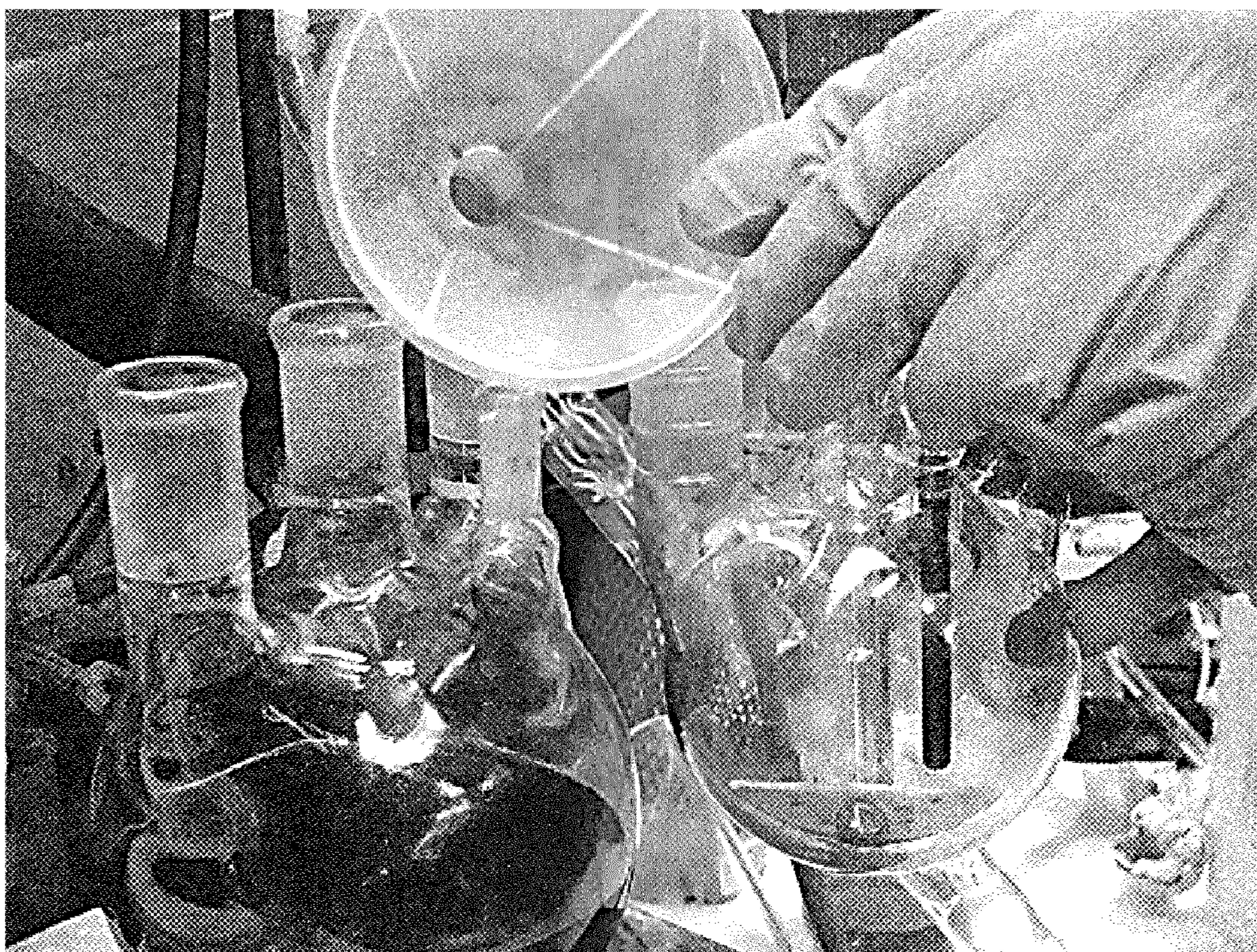
Figure 5: Reaction transfer of the composition of Process C using DIPEA as a base.
