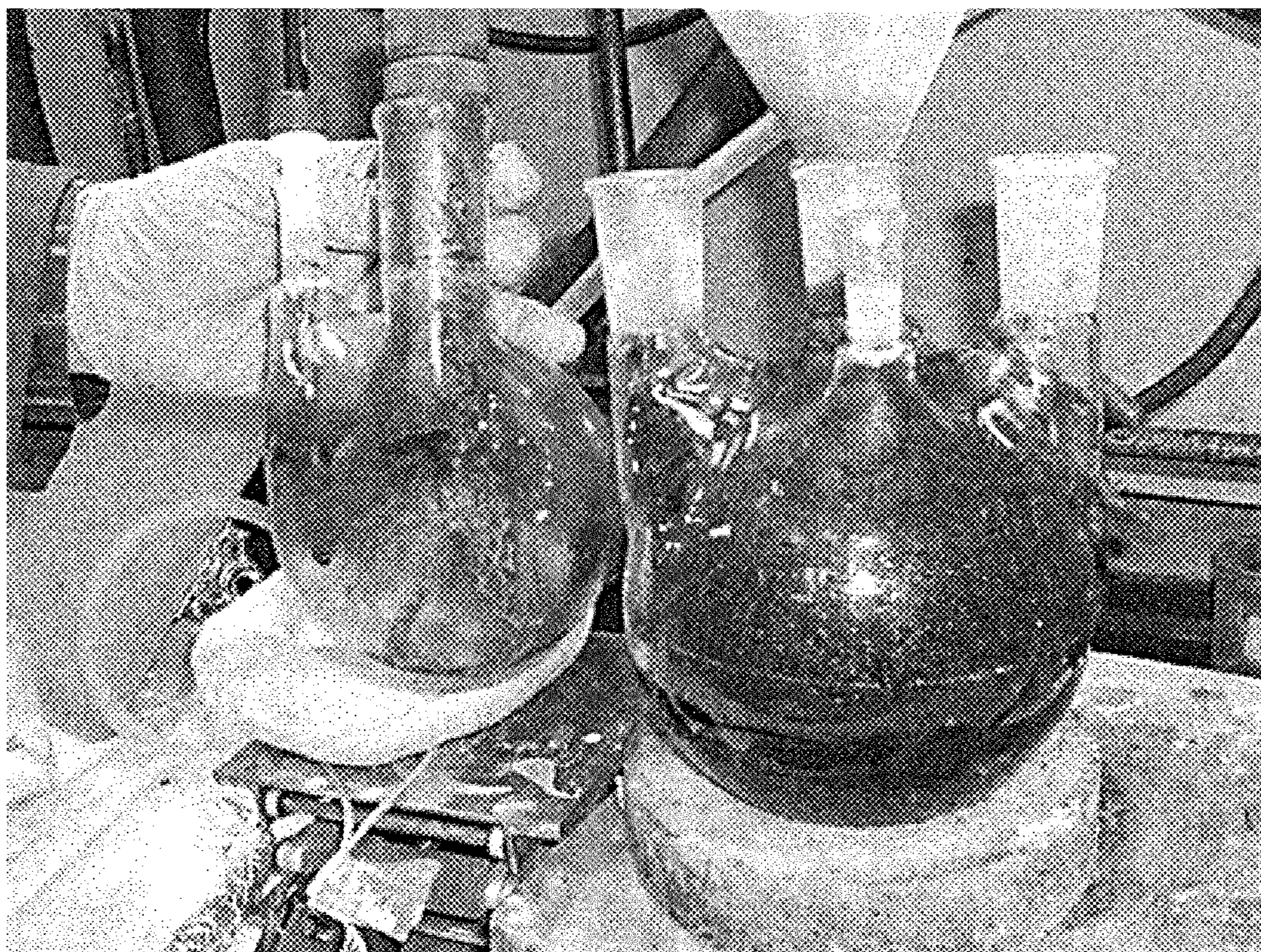
Figure 4: Reaction transfer of the composition of Step C using TEA as a base.
