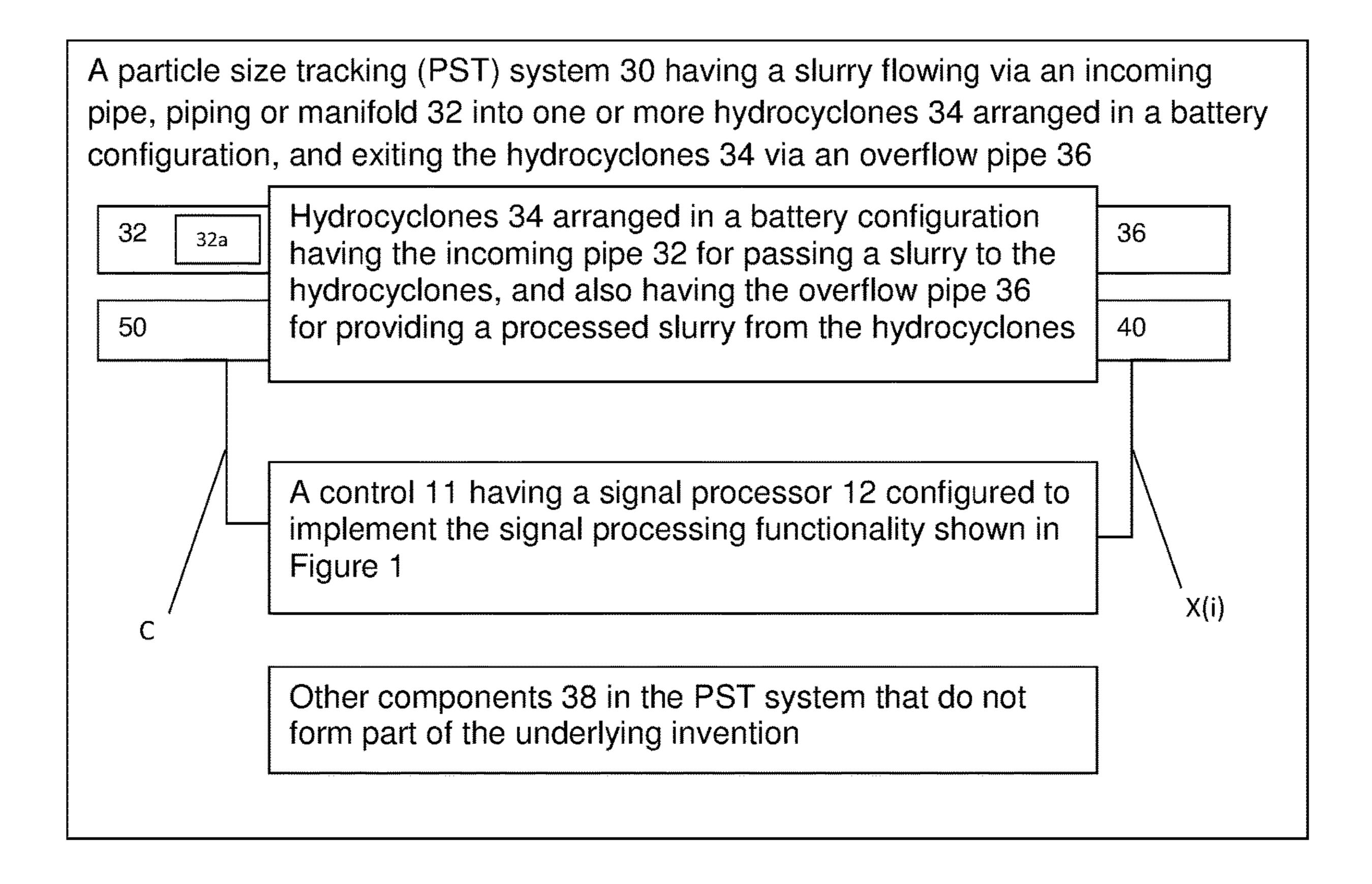
Figure 3: The Particle Size Tracking (PST) System 30
