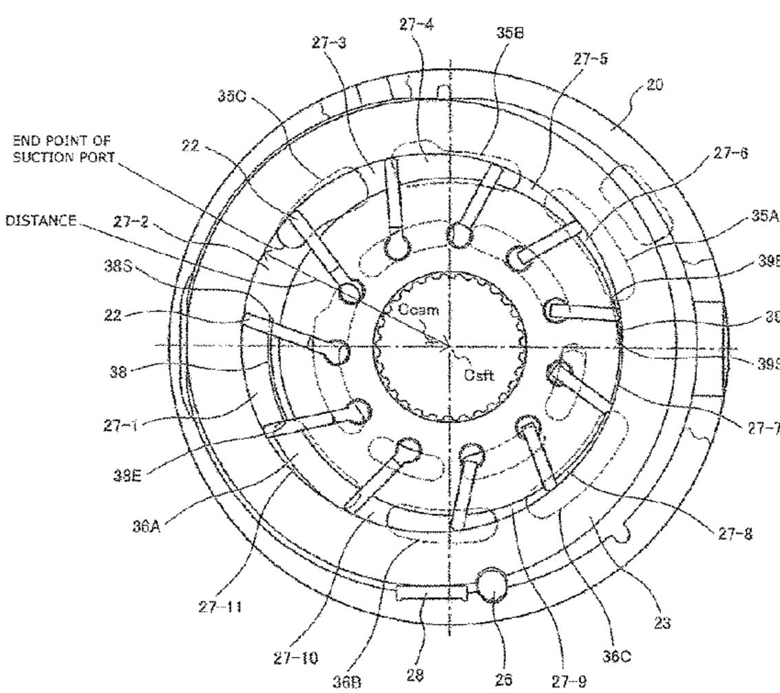
rear-side pump chamber (27-2) that communicates with the suction port (35), thereby lessening excessive pressure increase of the front-side pump chamber (27-1) and suppressing pulsation phenomenon.
