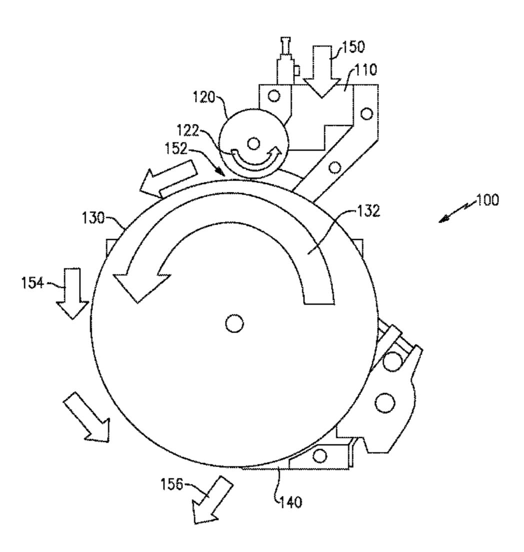
strip of edible material that is deposited on the cooling roller. The cooling roller then cools the strip of edible material and it is separated from the cooling roller by a blade. Once the strip is separated from the cooling roller it is deposited on a base of edible material such as a cookie or wafer.
