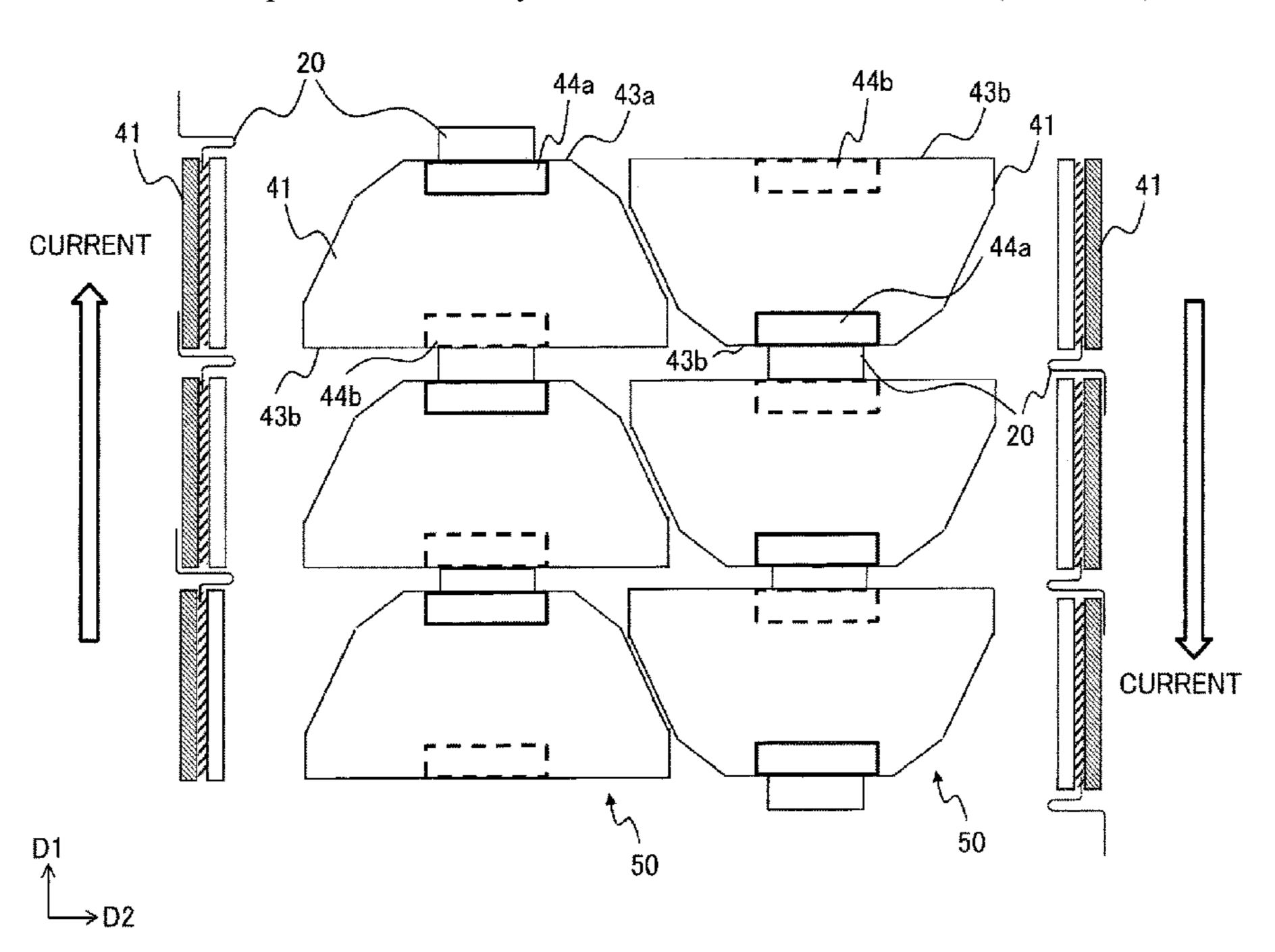
disposed in descending order of potential, with an end wider in width facing the one end (E1) in the first direction (D1), from the another end (E2) in the first direction (D1). Each of the plurality of first solar cell strings (51) and each of the plurality of second solar cell strings (52) are aligned alternately along the second direction (D2) that is orthogonal to the first direction (D1).
